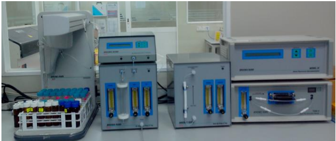
Figure 3.2: Automated – Gas Chromatography Cold Vapor Atomic Fluorescence Spectrometer
