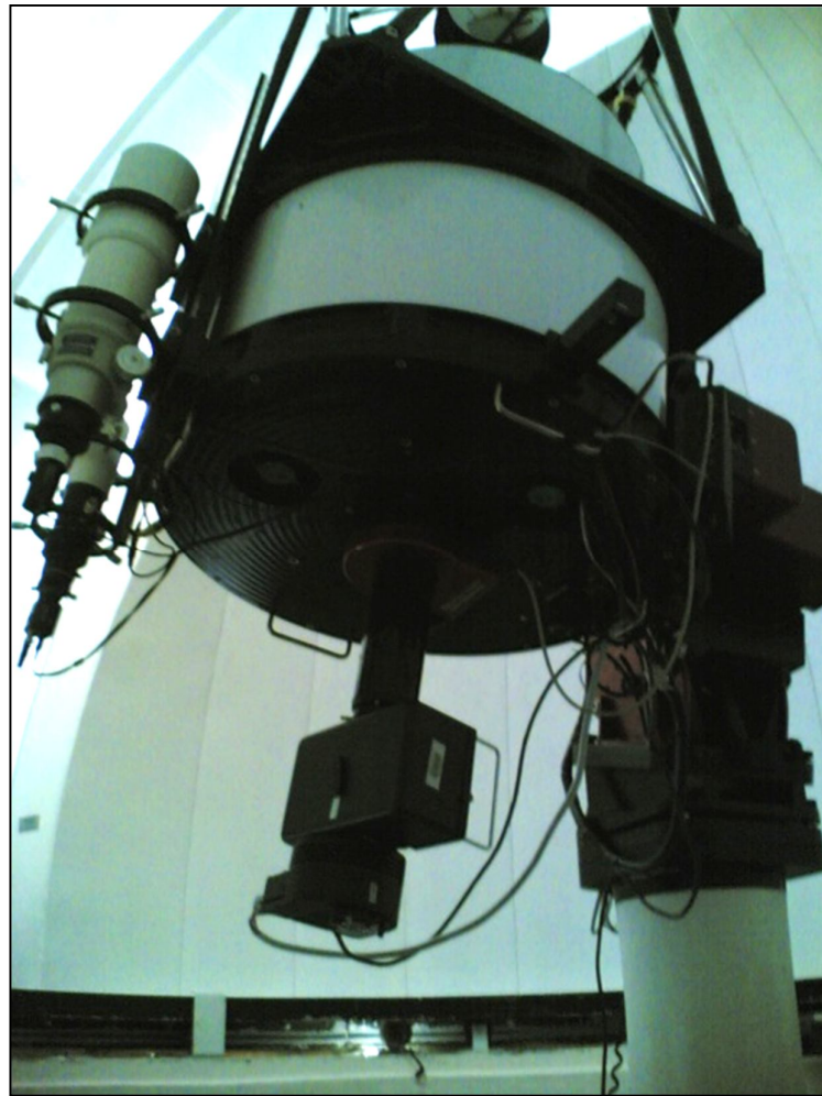
Figure 3.21: The telescope, the spectrograph and the CCD camera are all attached together in Langkawi National Observatory.
