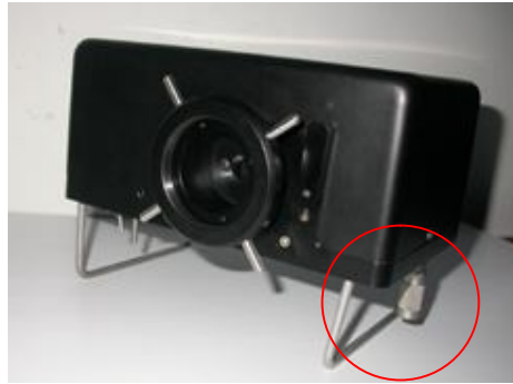
Figure 3.11: The micrometer screw outside the spectrograph.
