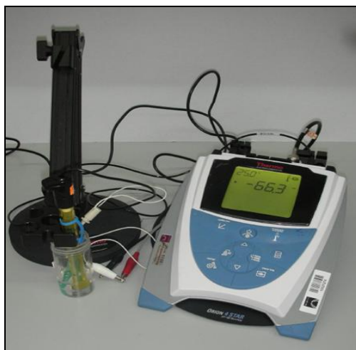
Figure 3.3: Measurement setup for ion-selective electrode potentiometric cell.
