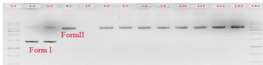
Figure 5.1: Topoisomerase I inhibition assay by gel electrophoresis for \text{H}_3\text{L}^1
