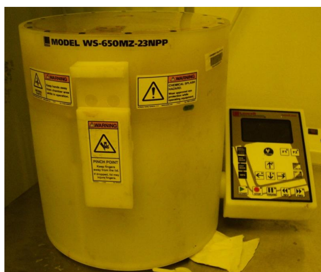
Figure 3.2 : Laurell WS-650MZ-23NPP spin coater.
