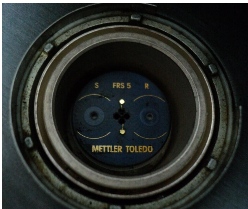
Figure 3.5: Two specific positions in the sample chamber. S and R represent as sample and reference position respectively.
