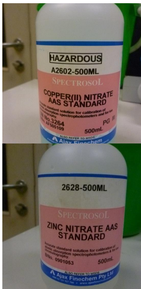
Figure 18: The copper stock standard (1000 ppm) that was used for making the standard solutions for the calibration curve.
