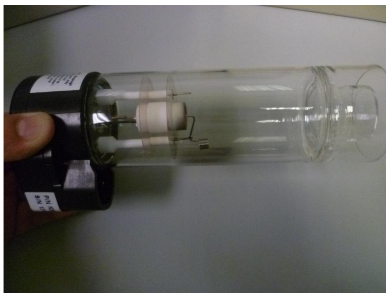
Figure 17: A hollow cathode lamp (HCL)
