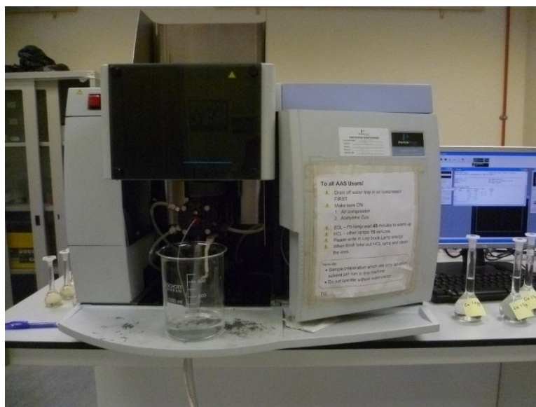
Figure 16: A Perkin Elmer AAnalyst 400 Atomic Absorption Spectrometer (AAS) that was used for the determination of trace metals in the crude oil samples.
