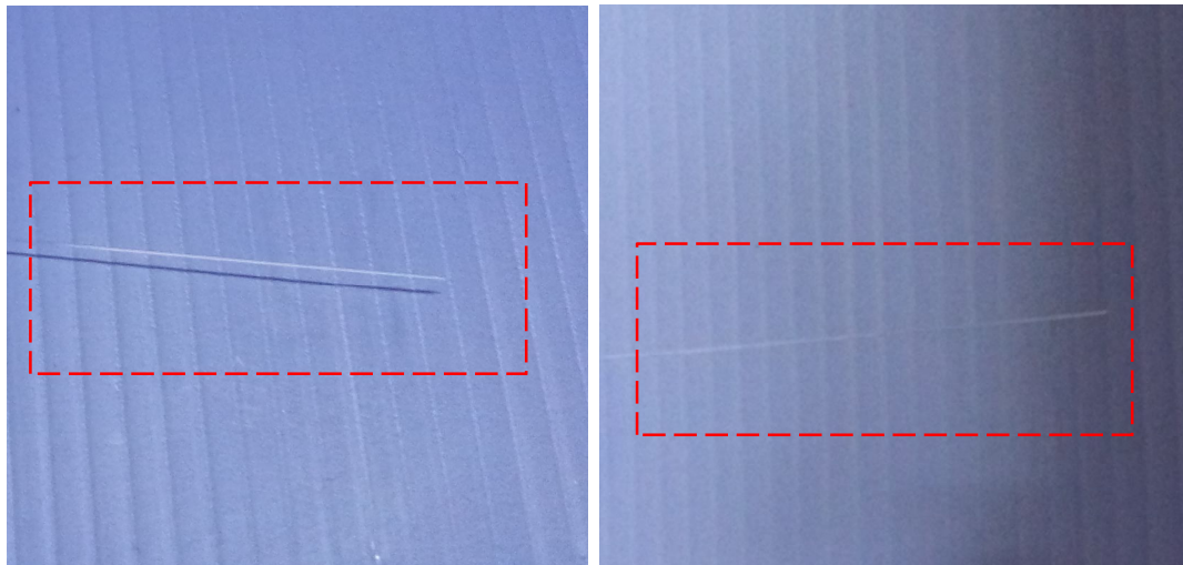
Figure 13: ZEr-A (above left) and ZEr-B (above right) (both highlighted by the red boxes) sample fibres as seen without any magnification. Due to the fibres being very thin, they are not easily visible, even when placed on a contrasting background. As such, the red box is used to highlight the fibres in the figures above.
