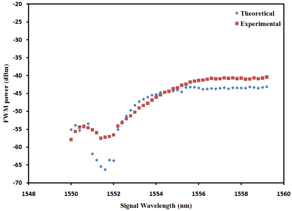
Figure 60: FWM conversion efficiency versus wavelength detuning 37 .
