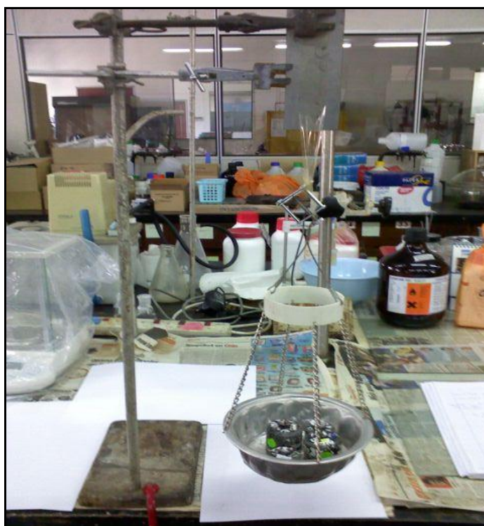
Figure 2.3: Apparatus set up for shear strength test
