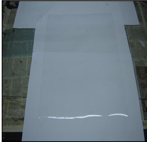
Figure 2.4: Tape underwent adhesive weight per unit area test.
