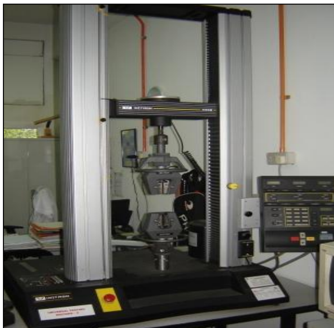
Figure 2.2: Instrument set up for peel strength test
