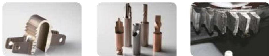
Figure 2.1: Example of products made using WEDM (source: AGIE Charmilles Group's website – www.gfac.com )
