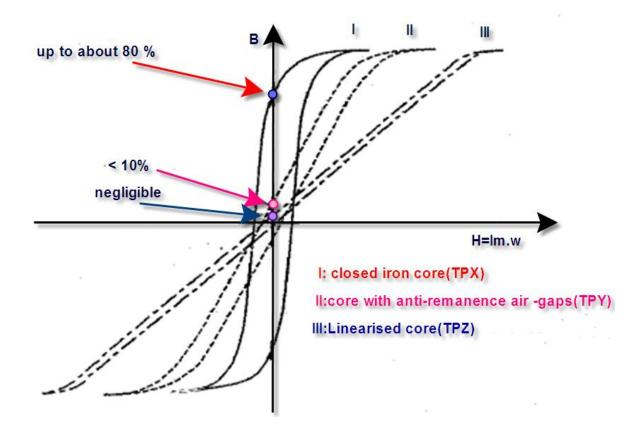
Figure 3.12 CT classes according to IEC 60044-6, magnetizing curves
