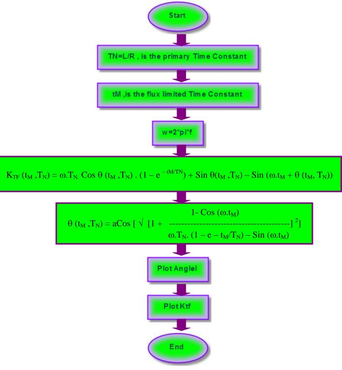
Figure 3.11 Flow chart of over dimensioning Factor  $K_T$
