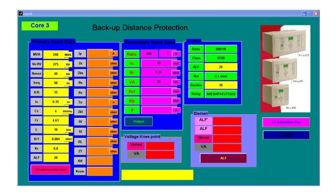
Figure 3.26 The General Layout Of GUI for Program of "Back Up Distance"
