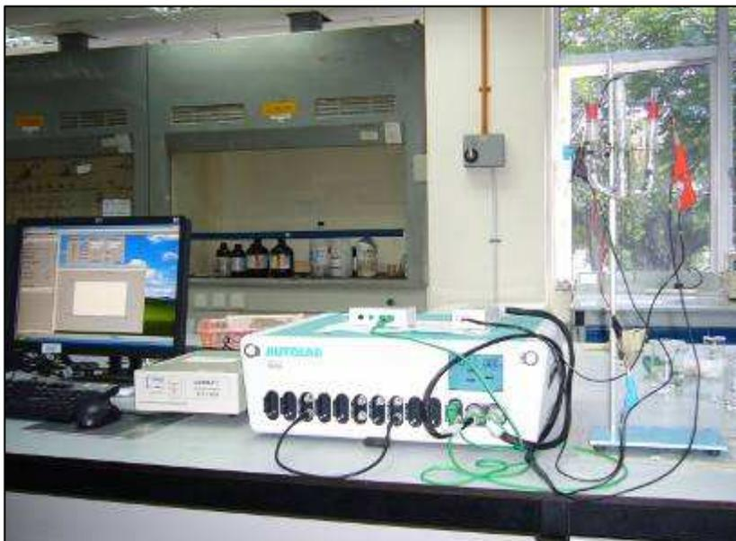
**Figure 3.16:** Cyclic voltammetry and Chronoamperometry experiments set up
