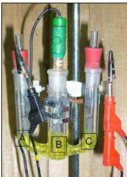
**Figure 3.17:** 3-electrode cell, A:Counter electrode, B:Reference electrode, C:Working electrode
