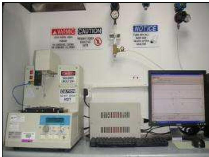
**Figure 3.13:** RHESCA SAT-5100 wetting balance gauge
