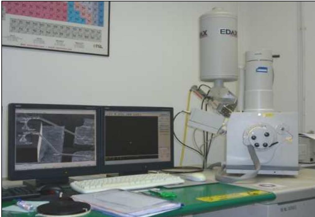
**Figure 3.4:** SEM and EDX: Philips XL and EDAX Analyzer Genesis
