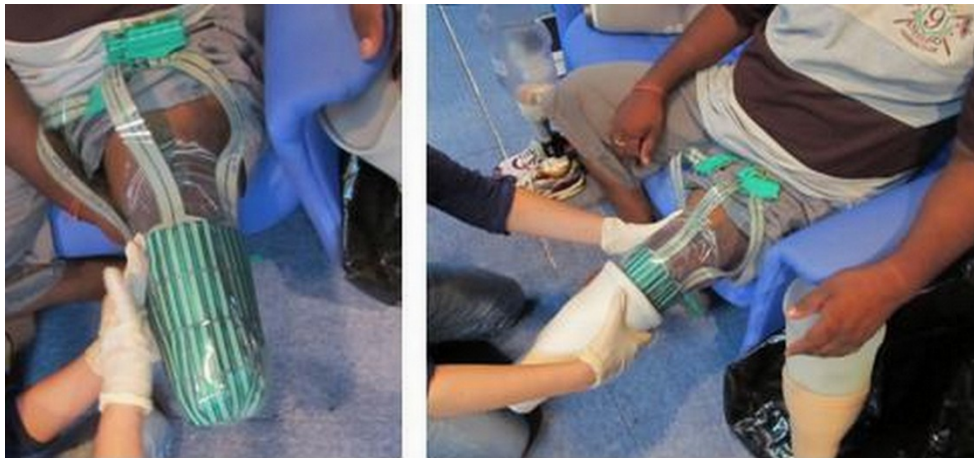
Figure 5.2: The sensor arrays mounted on the subject's residual limb.
