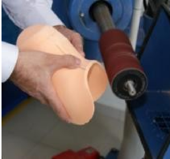
Figure 1.4: Pelite liner made of the polyethylene foam sheet used with the PTB socket.
