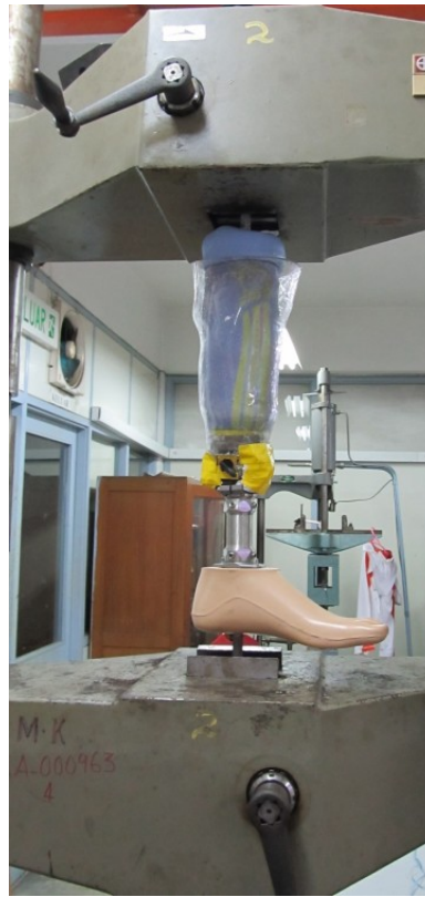
Figure 3.4: Mechanical testing. Tensile testing for the new prosthesis coupling system.
