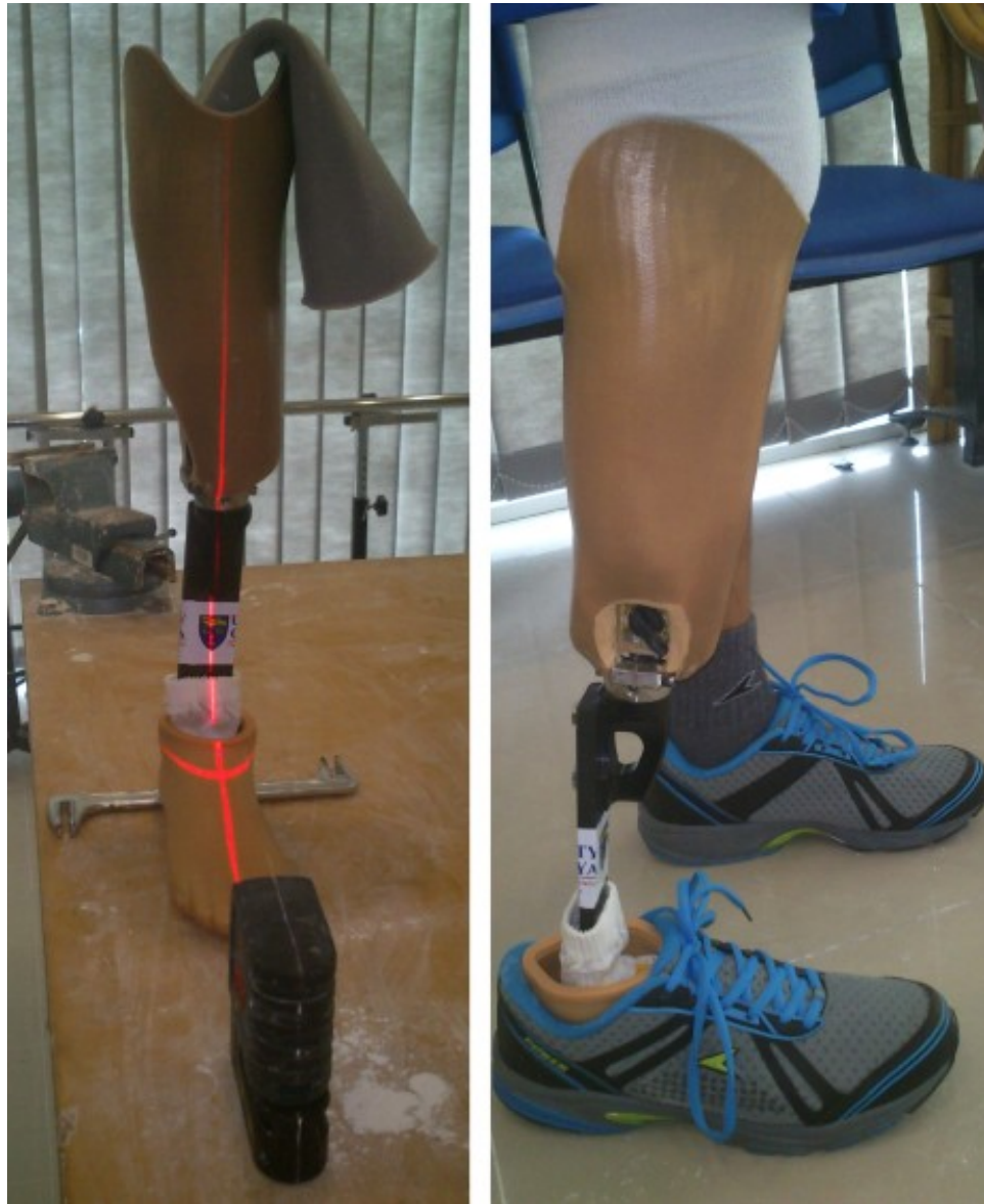
Figure 1.14: Bench and dynamic aligning of the definite prosthesis using the laser liner.
