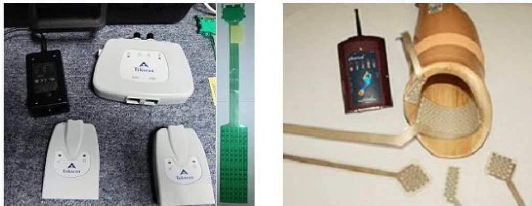
Figure 2.29: Transducers for in-socket pressure mapping; the Novel Pliance 16P System (Right; (Novel, 2014) and the Tekscan F-Socket system (Left).
