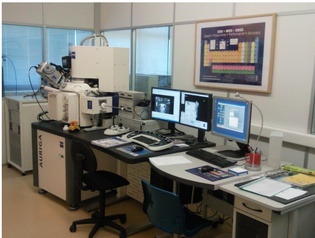
Figure 3.2 : Photo of Scanning electron microscope AURIGA cross Beam Workstation (FESEM laboratory, Faculty of Engineering, University of Malaya) .
