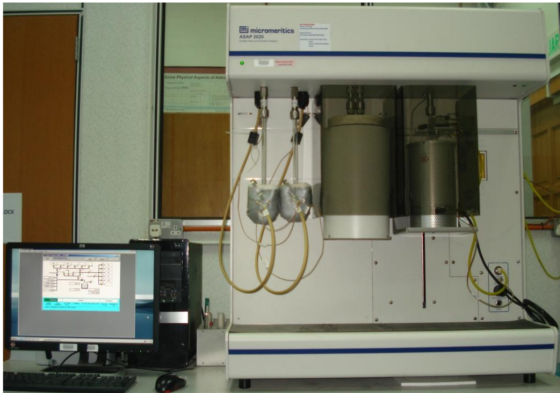
Figure 3.3 : Micromeritics ASAP 2020 surface area and porosity analyzer
