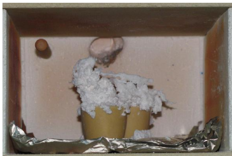
Figure 3.1: The expanded materials after calcination process because of gelatin.
