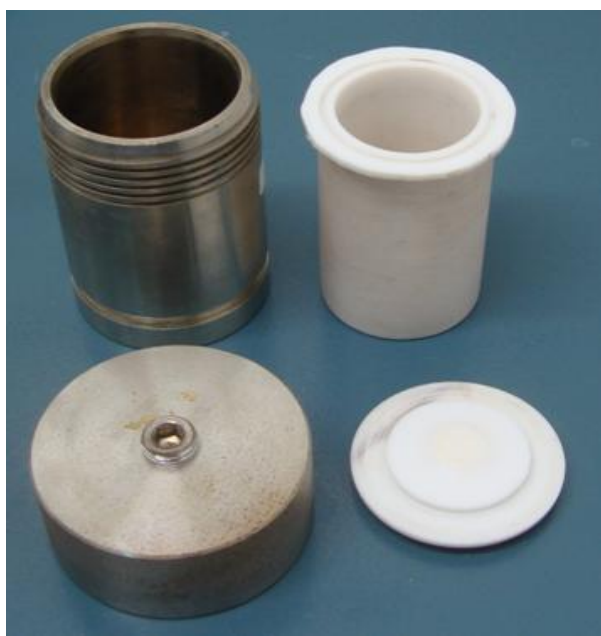
Figure 3.5: The autoclave and its Teflon vessel used for experiment.
