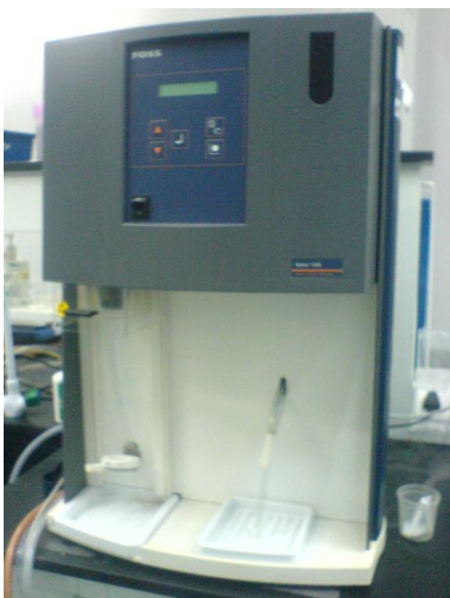
Appendix 1 (a); Figure 2: FOSS Tecator Digester Auto
