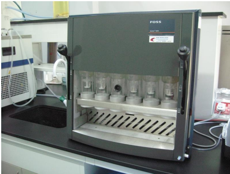
Appendix 1 (a); Figure 5: FOSS Soxtec 2055
