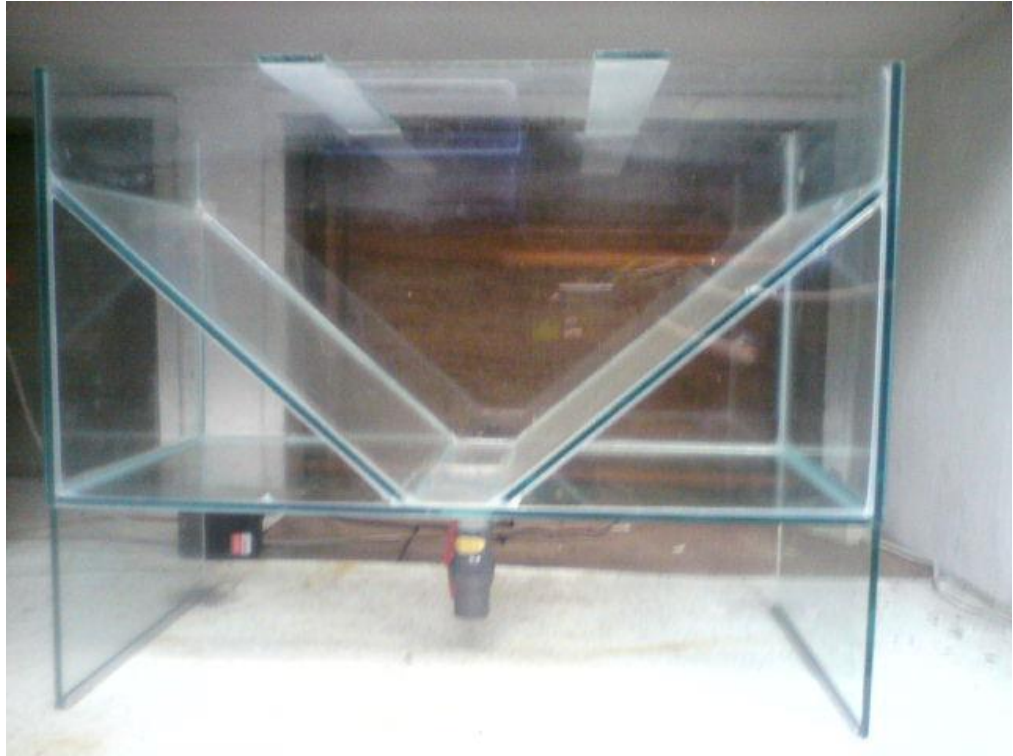
Figure 3.1: Modified 30L aquarium used for digestibility study
