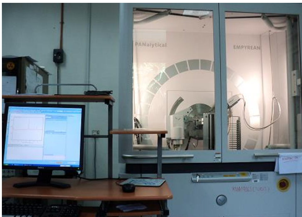
Figure 2.10: Schematic of XRD instrument
