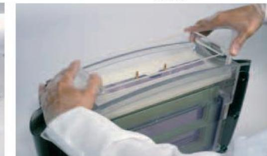
9 Sealing the upper buffer chamber.
