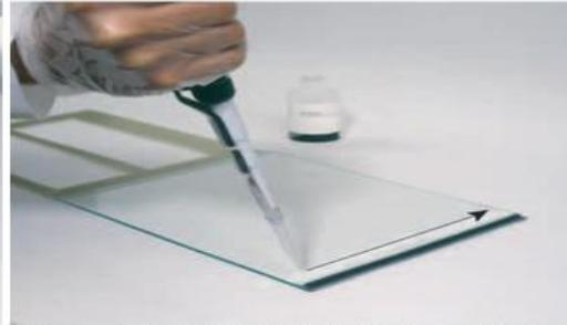
2 Pipetting a streak of gel buffer onto the glass plate. The arrow indicates the direction of motion in applying the streak.
