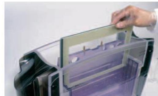
8 Inserting the cassettes into the cassette carrier.
