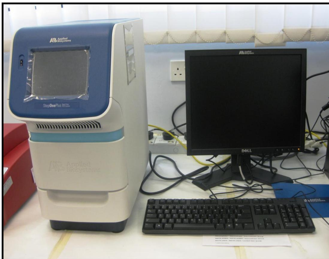
**Figure 5.3: Real- Time RT PCR (Applied Biosystem), with StepOne® 2.0 software.**
