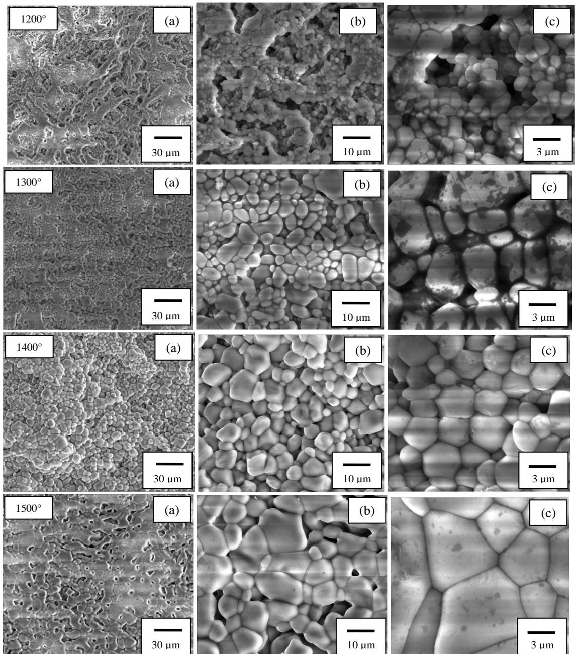
**Figure 4.36:** FESEM micrographs of forsterite compacts sintered at 1200°C, 1300°C, 1400°C and 1500°C with 1 hours holding time (Group 2)
