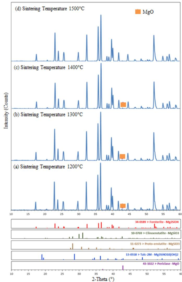
**Figure 4.10:** XRD traces sample set no.1 (3 hours ball milling and 1 hour heat treatment) after sintering at different temperatures (1200°C to 1500°C)
