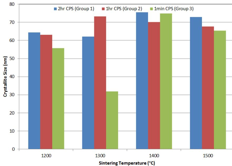
**Figure 4.24:** Crystallite size of forsterite produced with different sintering temperatures and holding times
