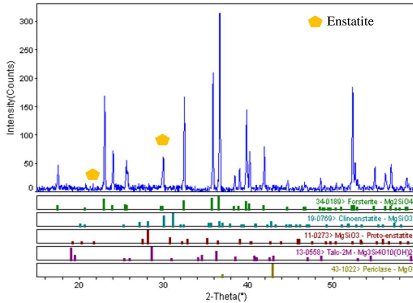
**Figure 4.22:** XRD traces of sintered forsterite compacts with 1400°C for 1 minute at 10°C/min
