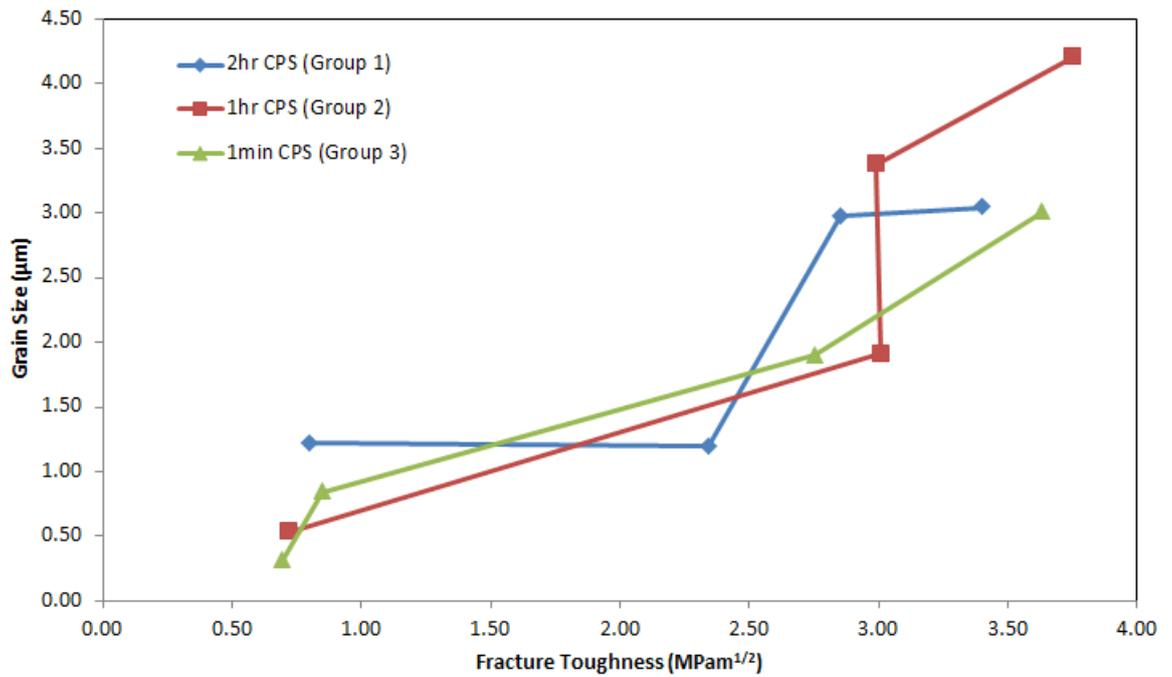
**Figure 4.44:** The effect of fracture toughness on grain size of sintered forsterite
