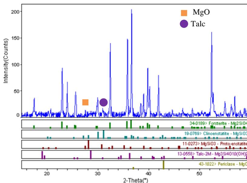
**Figure 4.20:** XRD traces of sintered forsterite compacts with 1200°C for 1 minute at 10°C/min
