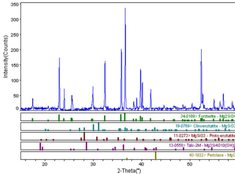
**Figure 4.19:** XRD traces of sintered forsterite compacts with 1500°C for 1 hour at 10°C/min
