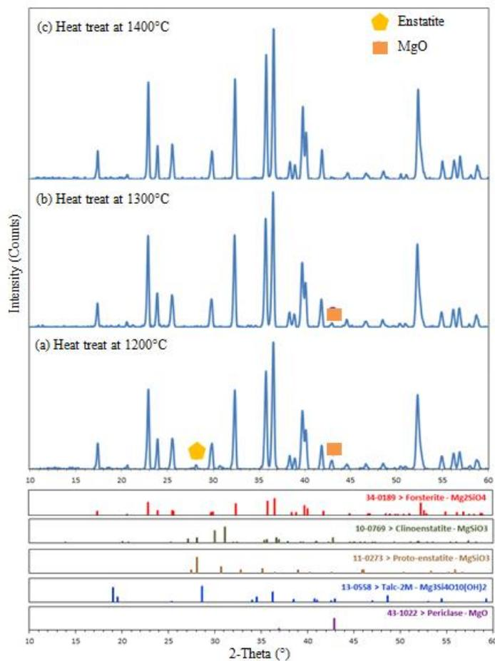
**Figure 4.8:** XRD traces of forsterite powder after ultrasonic bath, 3 hours ball milling and heat treatment at different temperature for 1 hour
