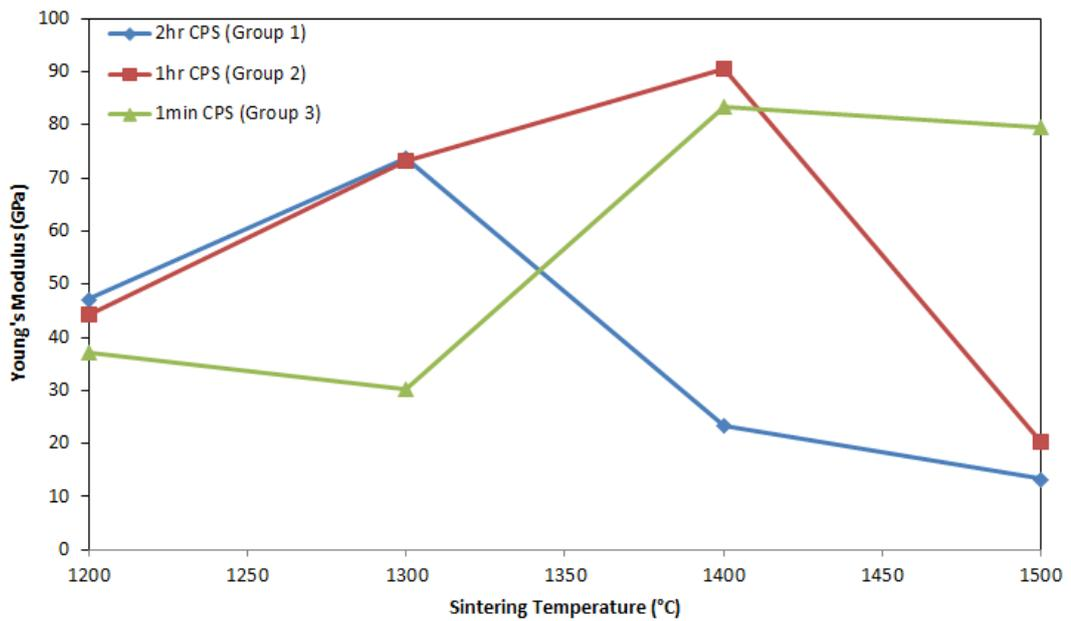
**Figure 4.33:** The effect of different sintering temperatures and holding times on Young's Modulus of forsterite
