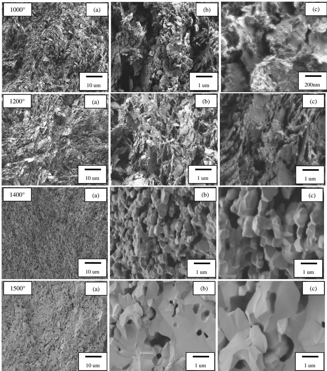
**Figure 4.39:** FESEM micrographs of cracked surface resulting from quenching after sintered at 1000°C, 1200°C, 1400°C, 1500°C with ramp rate of 10°C/min
