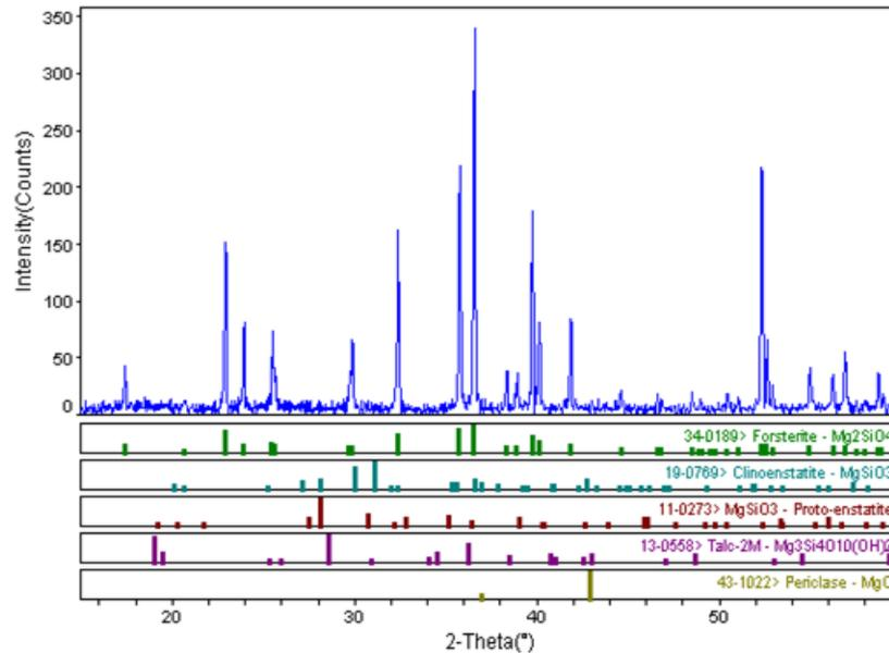
**Figure 4.14:** XRD traces of sintered forsterite compacts with 1400°C for 2 hours at 10°C/min
