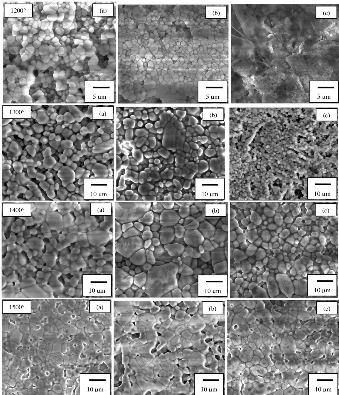
**Figure 4.38:** FESEM micrographs of sintered forsterite compacts sintered at 1200°C, 1300°C, 1400°C & 1500°C with 3 different holding times; (a) 2 hours (Group 1), (b) 1 hour (Group 2), (c) 1 minute (Group 3)
