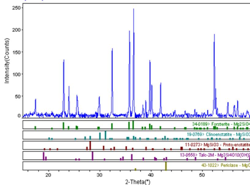
**Figure 4.16:** XRD traces of sintered forsterite compacts with 1200°C for 1 hour at 10°C/min
