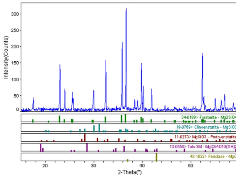
**Figure 4.23:** XRD traces of sintered forsterite compacts with 1500°C for 1 minute at 10°C/min
