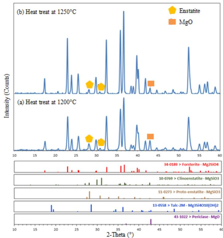
**Figure 4.7:** XRD traces of forsterite powder after 3 hours ball milling and heat treatment (1200°C & 1250°C) for 2 hours
