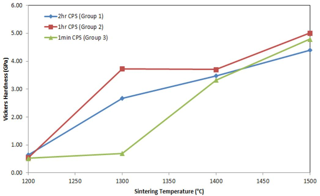
**Figure 4.29:** The effect of sintering temperature and holding time on Vickers hardness of forsterite samples
