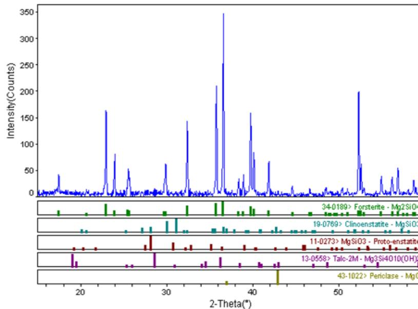
**Figure 4.15:** XRD traces of sintered forsterite compacts with 1500°C for 2 hours at 10°C/min
