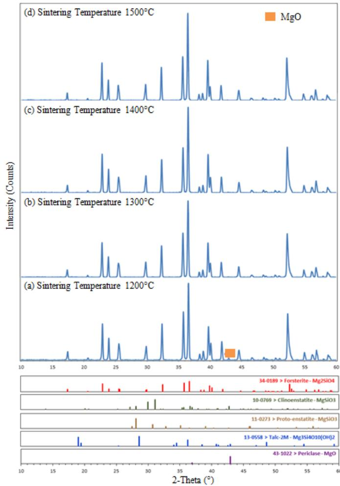
**Figure 4.11:** XRD traces sample set no.2 (3 hours ball milling and no heat treatment) after sintering at different temperatures (1200°C to 1500°C)
