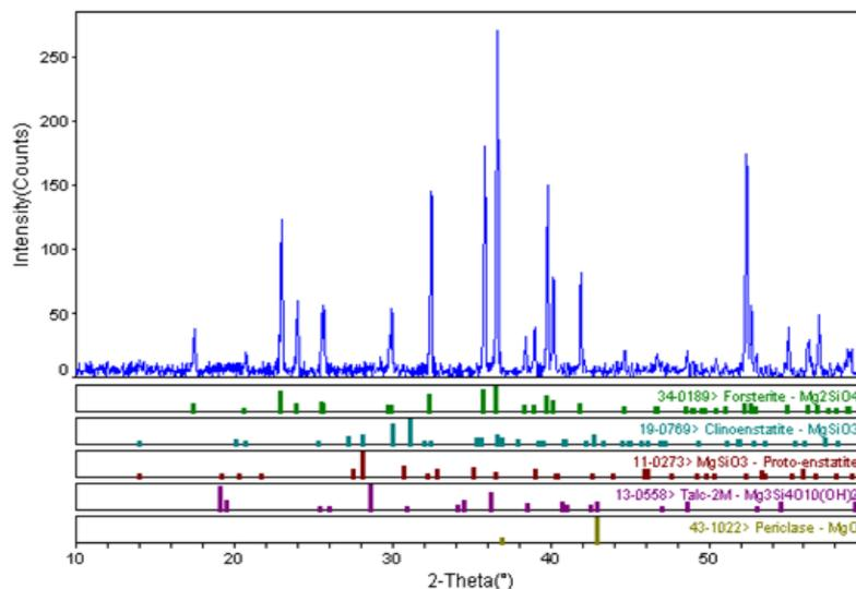
**Figure 4.12:** XRD traces of sintered forsterite compacts with 1200°C for 2 hours at 10°C/min
