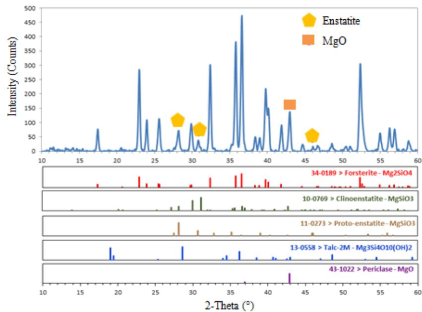
**Figure 4.2:** XRD traces of forsterite powder subject to 2 hours direct ultrasonification with 30% amplitude and 2 hours heat treatment at 1200°C
