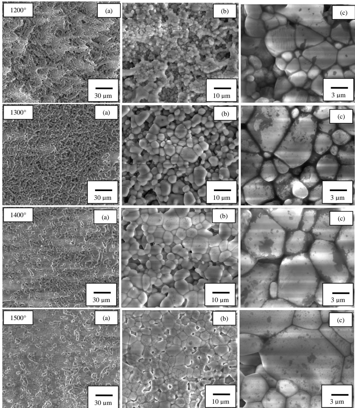
**Figure 4.35:** FESEM micrographs of forsterite compacts sintered at 1200°C, 1300°C, 1400°C and 1500°C with 2 hours holding time (Group 1)
