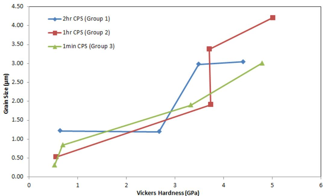
**Figure 4.43:** The effect of Vickers hardness on grain size of sintered forsterite
