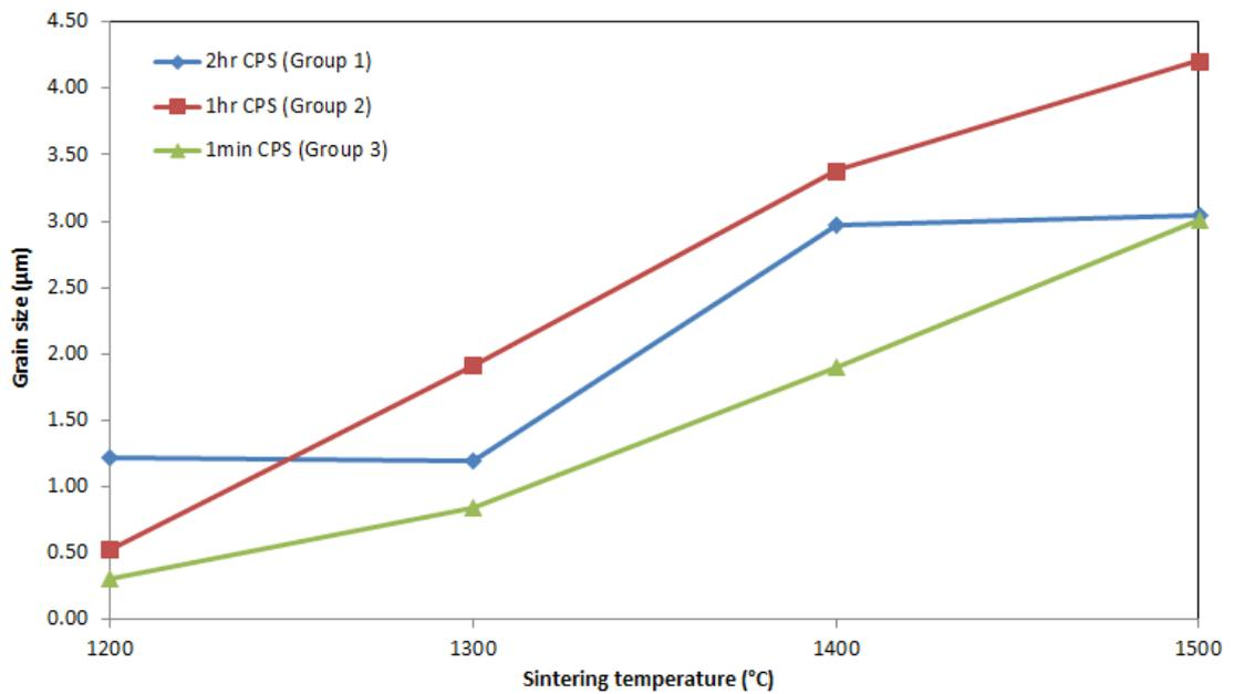
**Figure 4.41:** The effect of sintering temperature with three different holding times (Group1: 2 hours, Group 2: 1 hour and Group 3: 1 minute) on grain size of sintered forsterite compacts
