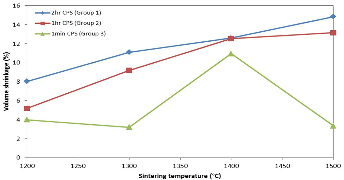
**Figure 4.25:** The effect of sintering temperatures and holding times on forsterite volume shrinkage
