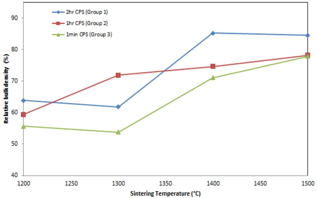
**Figure 4.26:** The effect of sintering temperatures and holding times on forsterite relative bulk density
