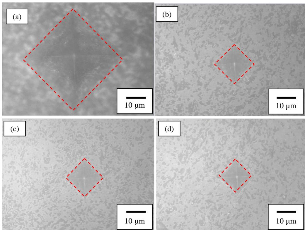
**Figure 4.27:** Diamond shaped Vickers indentation of forsterite sample sintered at 1200°C, 1300°C, 1400°C and 1500°C with 1 hour holding time
