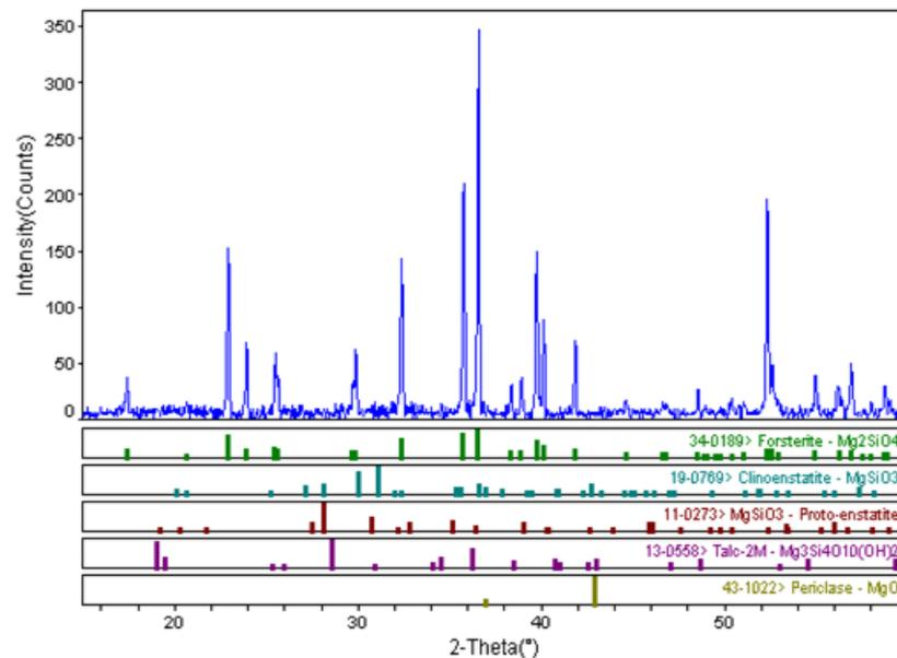
**Figure 4.13:** XRD traces of sintered forsterite compacts with 1300°C for 2 hours at 10°C/min
