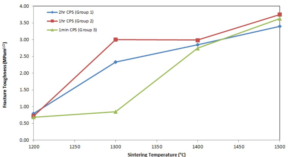
**Figure 4.31:** The effect of sintering temperatures and holding times on fracture toughness of forsterite compacts
