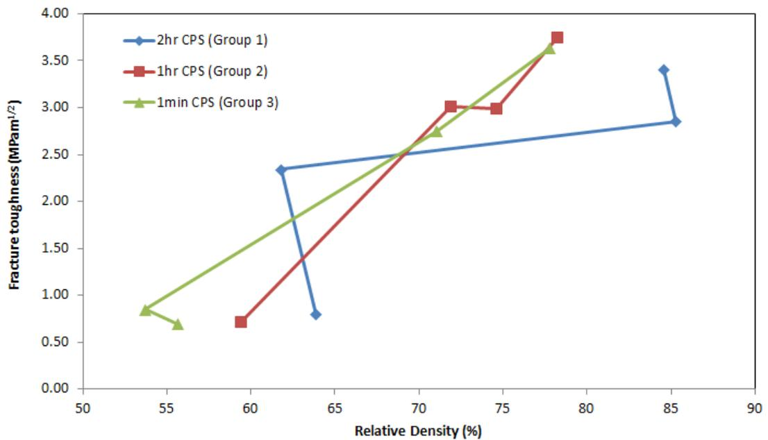
**Figure 4.32:** The effect of relative density on fracture toughness with different sintering temperature and holding time
