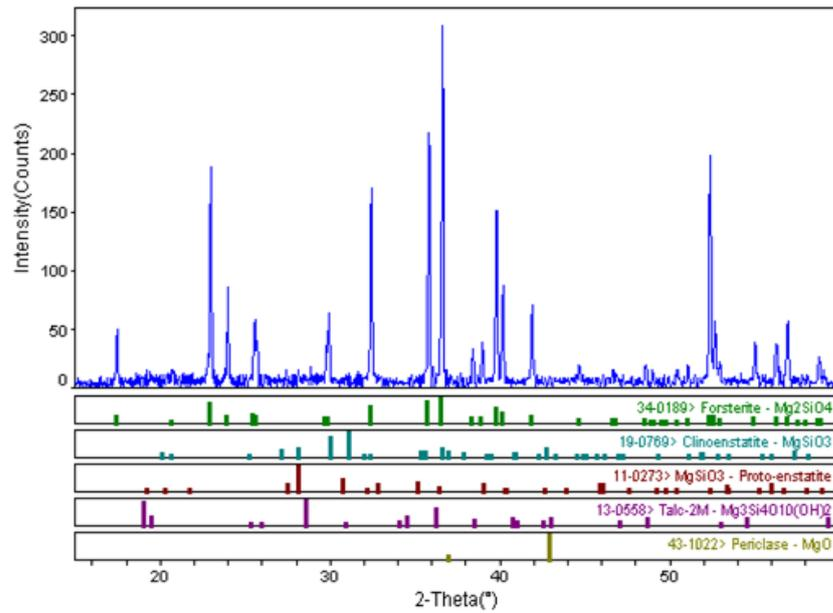
**Figure 4.17:** XRD traces of sintered forsterite compacts with 1300°C for 1 hour at 10°C/min
