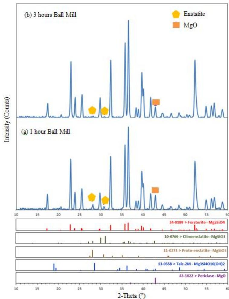
**Figure 4.4:** XRD traces of forsterite powder after direct ultrasonification with 30% amplitude and ball milling at various time after heat treatment
