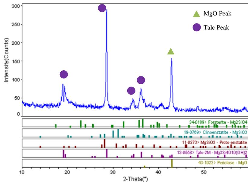
**Figure 4.1:** XRD traces of synthesized forsterite powder before sintering
