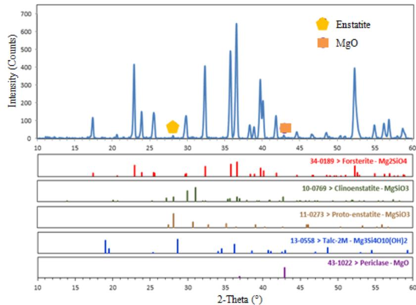
**Figure 4.6:** XRD traces of forsterite powder after direct ultrasonication with 50% amplitude, 3 hours ball milling and heat treatment 1250°C for 2 hours
