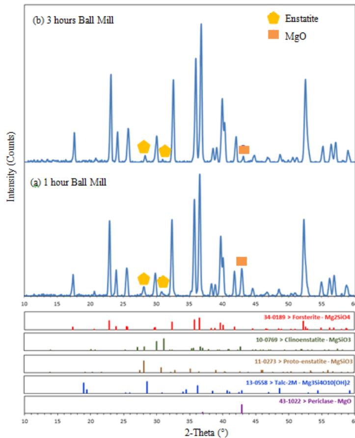
**Figure 4.5:** XRD traces of forsterite powder after direct ultrasonification with 50% amplitude and ball milling at various time after heat treatment
