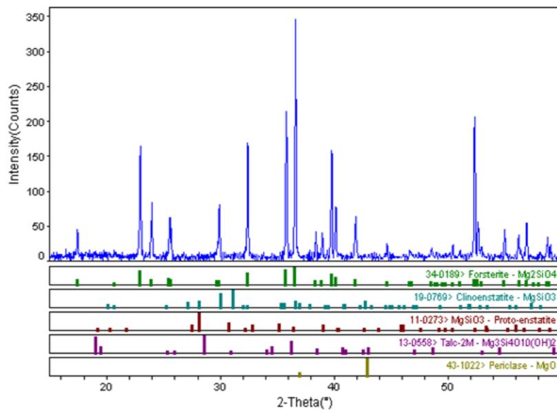
**Figure 4.18:** XRD traces of sintered forsterite compacts with 1400°C for 1 hour at 10°C/min
