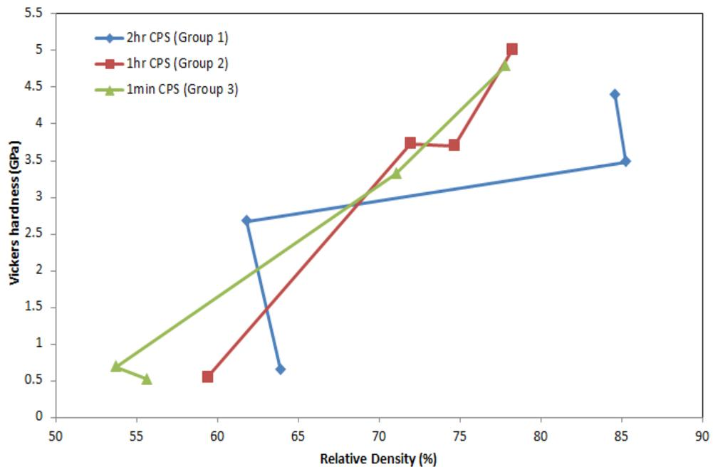
**Figure 4.30:** The effect of relative density on Vickers hardness with different sintering temperature and holding time
