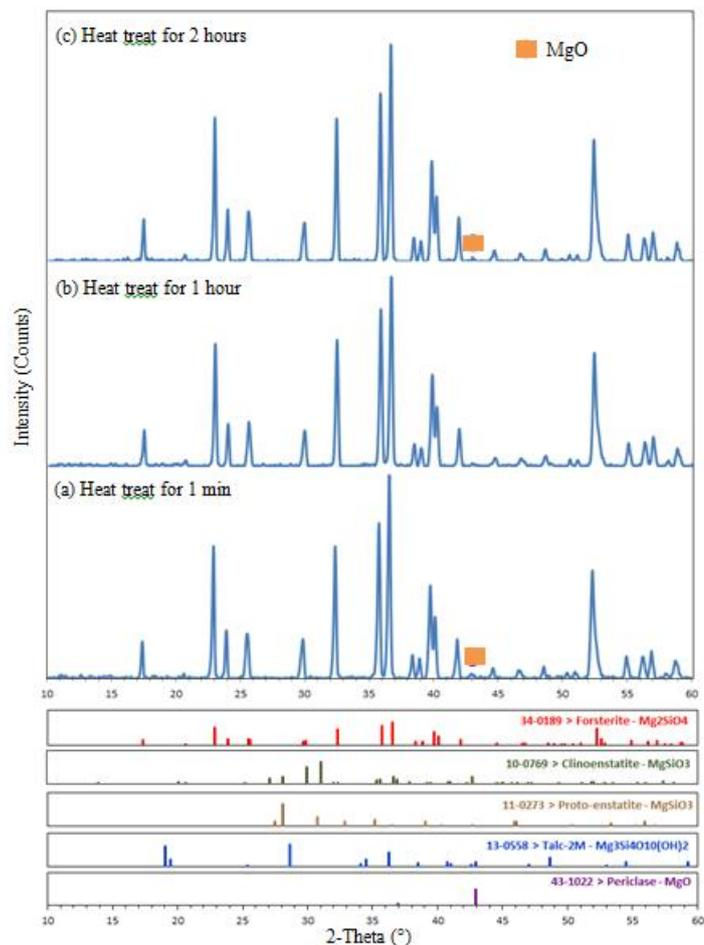
**Figure 4.9:** XRD traces of forsterite powder after 3 hours ball milling and 1 hour heat treatment at 1400°C with different holding time
