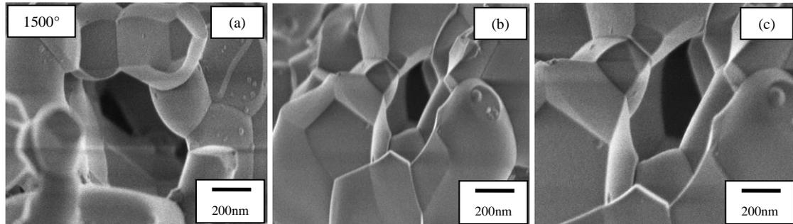
**Figure 4.40:** Closed up FESEM micrographs of forsterite compact sintered at 1500°C
