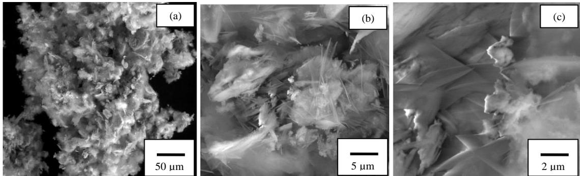
**Figure 4.34:** FESEM micrographs of forsterite powder prepared by 22 minutes ultrasonification and 3 hours ball milling
