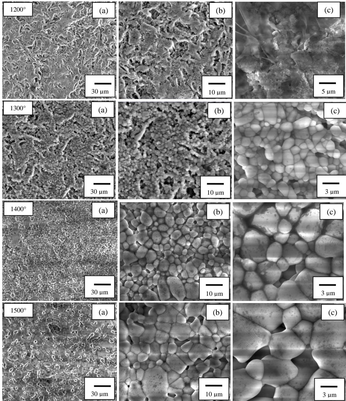
**Figure 4.37:** FESEM micrographs of forsterite compacts sintered at 1200°C, 1300°C, 1400°C and 1500°C with 1 minute holding time (Group 3)
