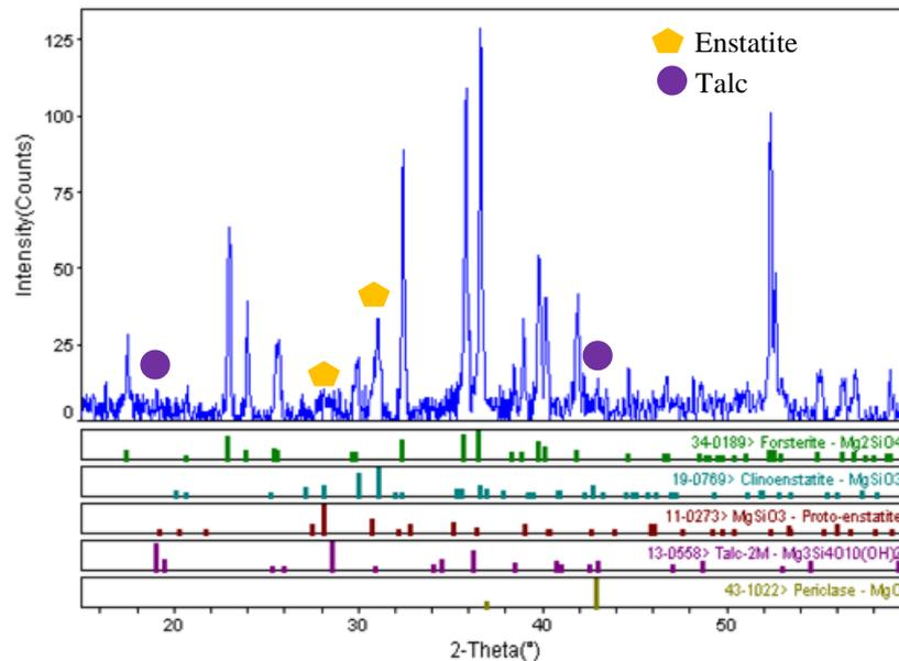
**Figure 4.21:** XRD traces of sintered forsterite compacts with 1300°C for 1 minute at 10°C/min
