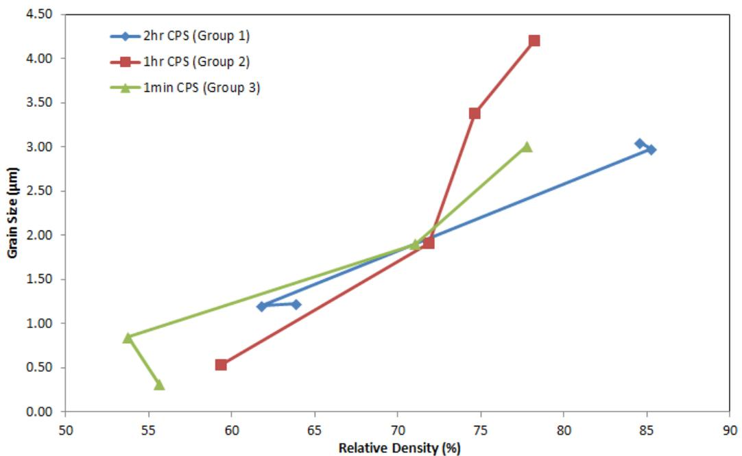
**Figure 4.42:** The effect of relative density on grain size of sintered forsterite with
