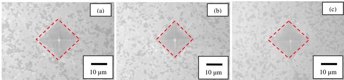
**Figure 4.28:** Diamond shaped Vickers indentation of forsterite sample sintered at 1500°C with 3 different holding times; (a) 2 hours, (b) 1 hour, (c) 1 minute
