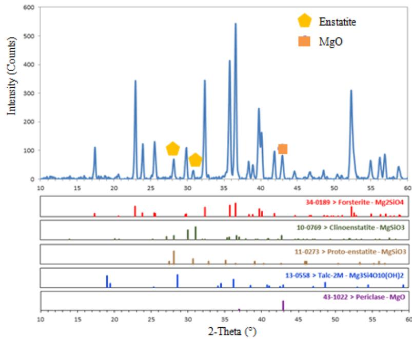
**Figure 4.3:** XRD traces of forsterite powder subject to 2 hours direct ultrasonication with 50% amplitude and 2 hours heat treatment at 1200°C
