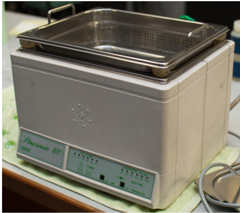
Figure C-5: Liarre ultrasonic bath machine
