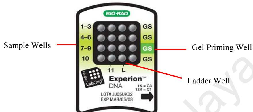
Figure 3.3: Experion DNA chip 1K. The locations of the gel priming well (GS, highlighted) and alphanumeric priming codes are indicated.
