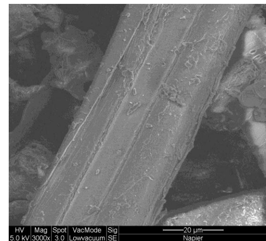
Fig. 4.44 SEM image of treated Napier fibers at 3000x magnification
