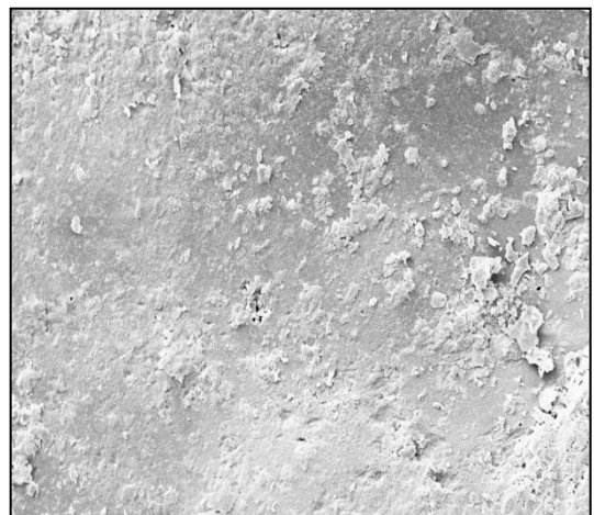
Fig. 4.231 SEM micrograph of PVA/1RS/3BB film surface after 2 weeks of outdoor burial
