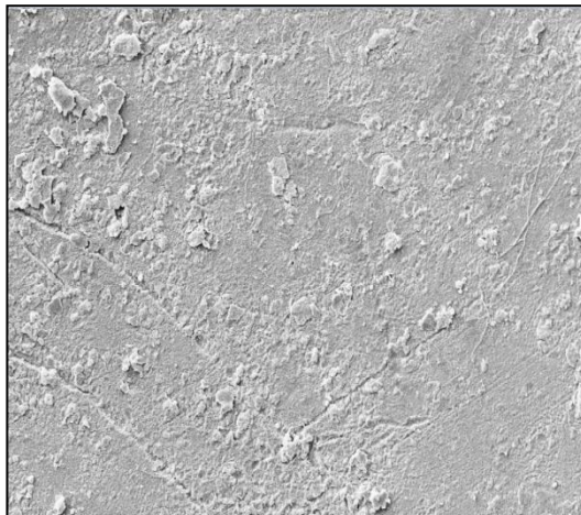
Fig. 4.228 SEM micrograph of PVA/1RS/1BB film surface after 2 weeks of indoor burial
