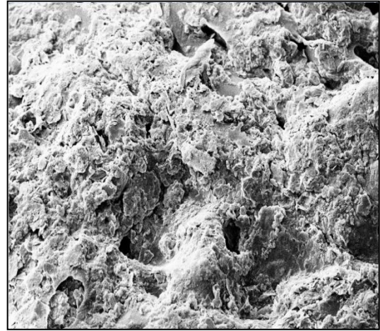
Fig. 4.245 SEM micrograph of PVA/1SS/1BB film surface after 2 weeks of outdoor burial
