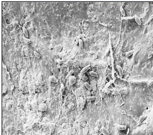
Fig. 4.234 SEM micrograph of PVA/1RS/3KF film surface after 2 weeks of indoor burial
