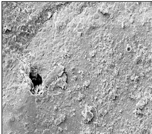
Fig. 4.252 SEM micrograph of PVA/1SS/1ROS film surface after 2 weeks of indoor burial
