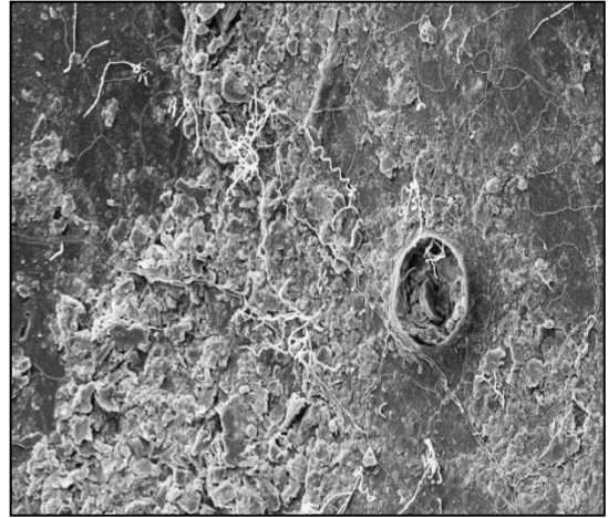
Fig. 4.215 SEM micrograph of PVA/1TS/3BB film surface after 2 weeks of outdoor burial
