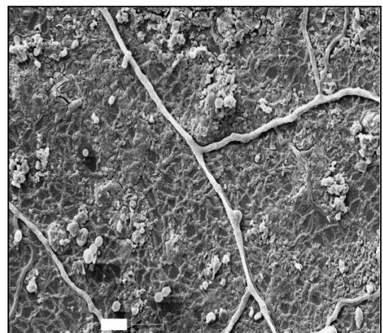
Fig. 4.195 SEM micrograph of PVA/ITS film surface after 2 weeks of outdoor burial
