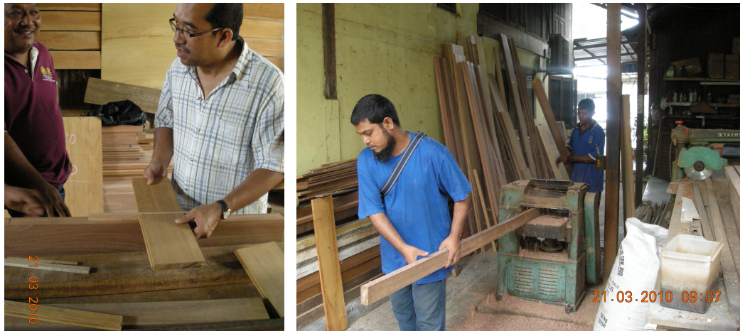
Figure 5.31: Manufacturing Prototype of RTA Components in a Local Carpenter's Workshop
