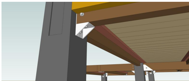
Figure 5.17: Steel Brackets Located at Lower Column to Receive Floor Beams
