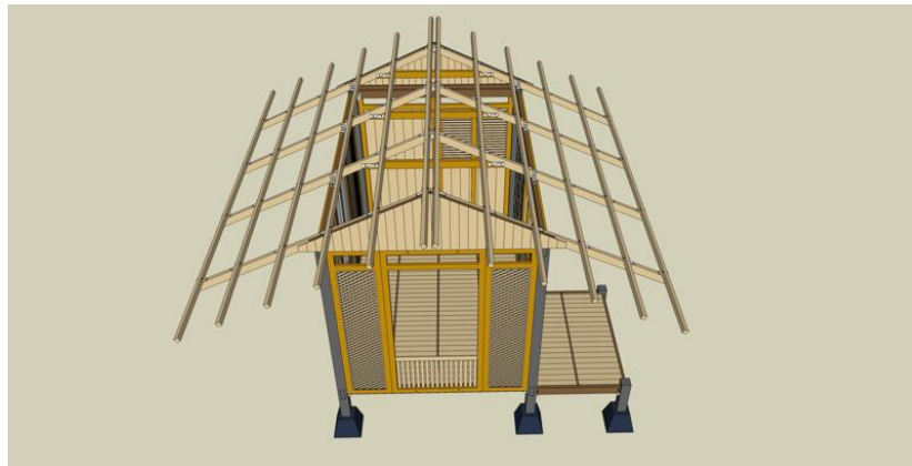
Figure 5.24: Roof Battens are Placed Accordingly to the Brackets Pre-Fixed on the Trusses
