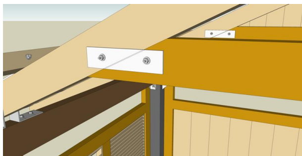
Figure 5.28: Connectors for Roof Trusses
