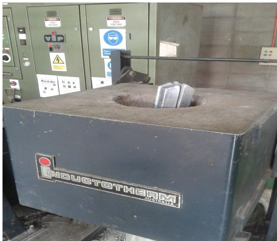
Figure 3.3: Induction furnace for melting ingot
