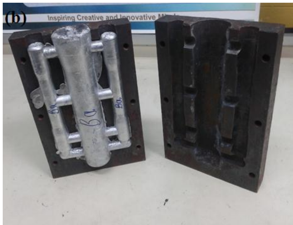
Figure 3.6: (a) Impact test and (b) tensile test samples permanent mold.
