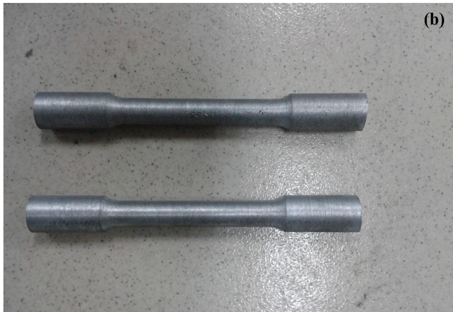
Figure 3.7: (a) Impact test and (b) Tensile test samples.
