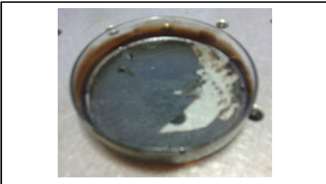
Figure 5.9: Image of the GO 'paper' obtained through filtration.
