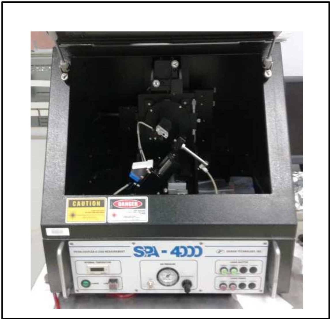
Figure 6.1: Sairon Technology SPA-4000 Prism Coupler available at the Class 10K Cleanroom of Photonics Research Centre, University of Malaya.
