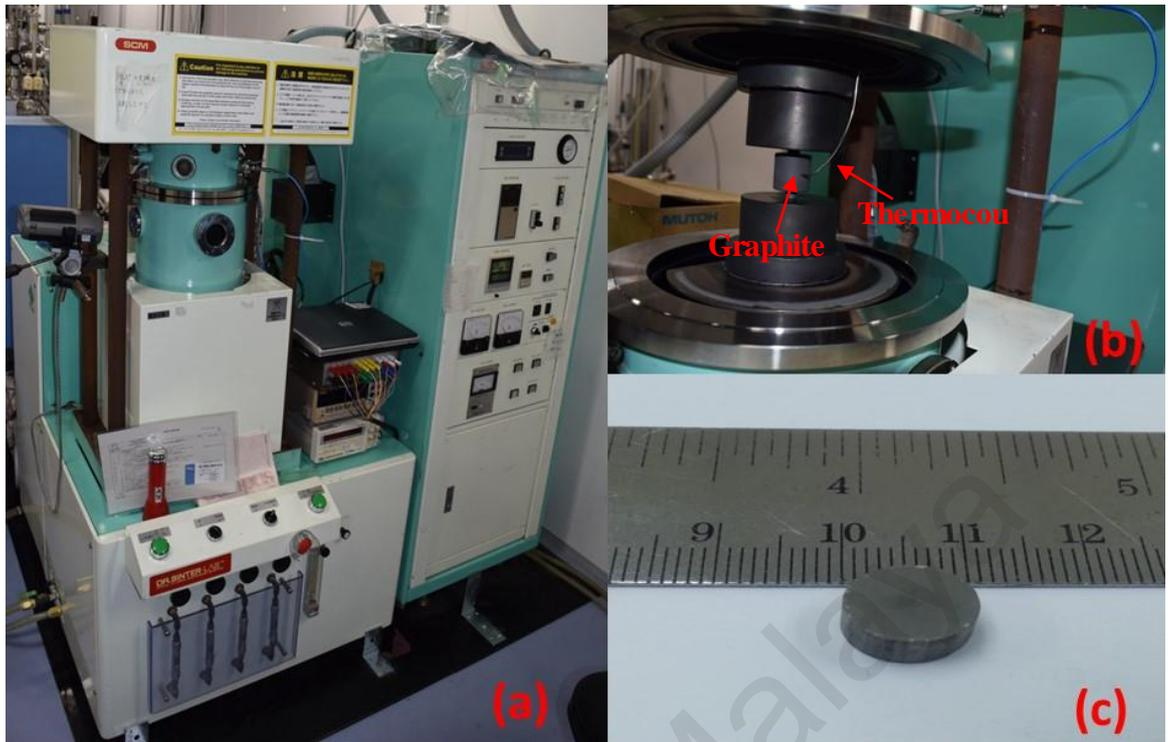
**Figure 3.2:** (a) Spark plasma sintering (SPS) system, (b) graphite die inside the chamber, and (c) the final disc shape after the SPS process.
