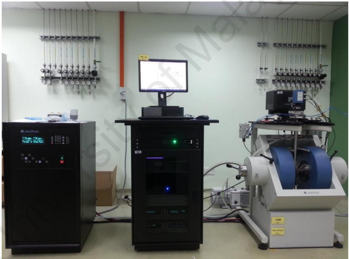
**Figure 3.10:** The Lake Shore 8400 Series instrument for Hall mobility measurement.
