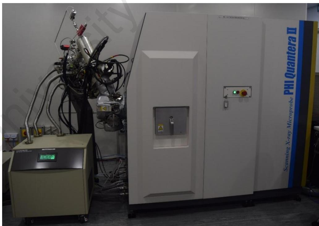
**Figure 3.6:** X- photoelectron spectroscopy (XPS) from Ulvac Phi (model: Quanterra II).
