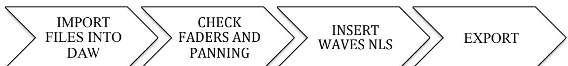
Figure 3.8: Diagram of the digital summing procedures with Waves NLS
