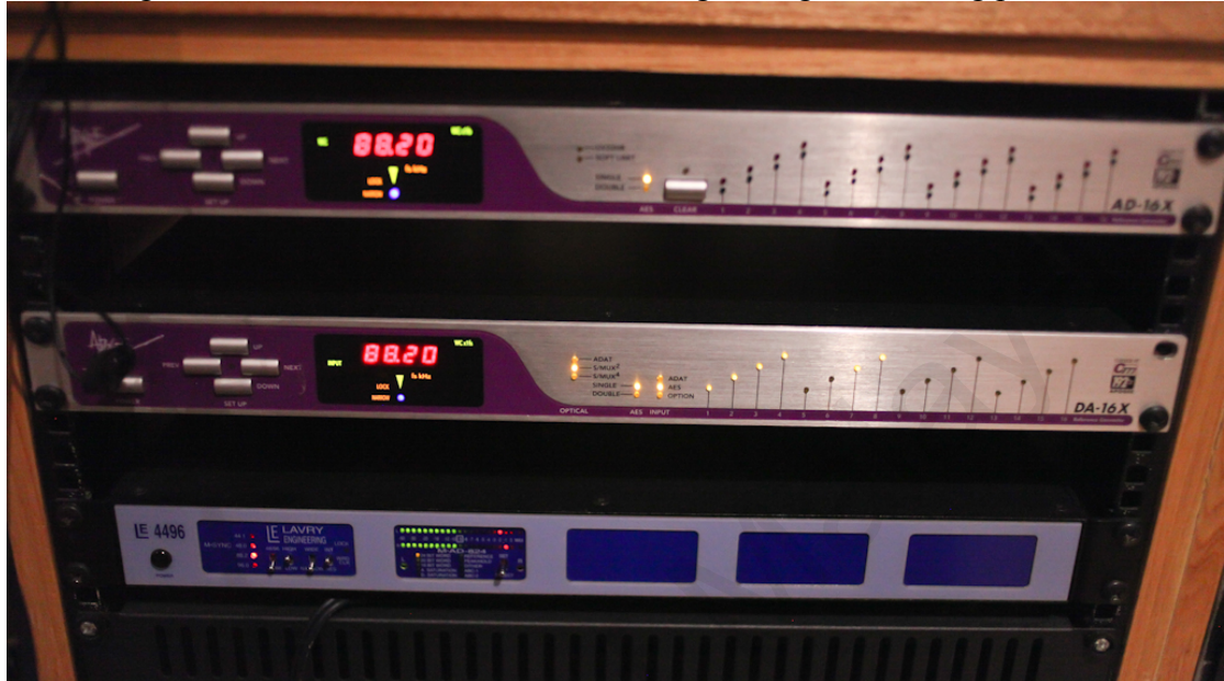
Figure 3.5: AD/DA converters used during analogue summing procedures
