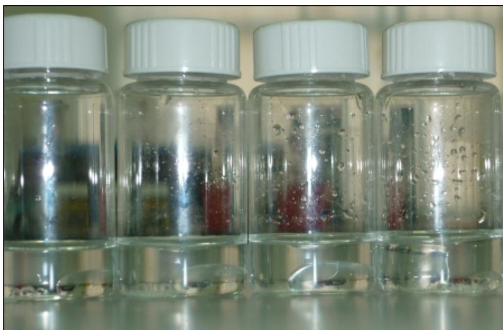
Figure 4.7: Mixture of dichloromethane, Cyanex923 and phenol solution (from left to right: increase in Cyanex923 concentration)
