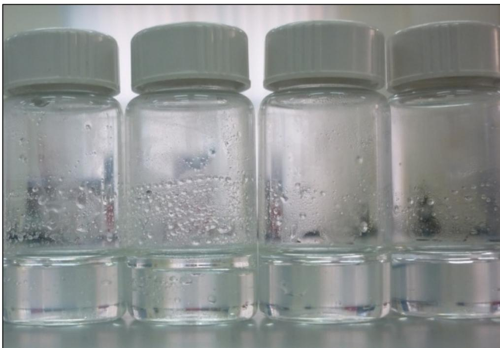
Figure 4.6: Mixture of kerosene, Cyanex923 and phenol solution (from left to right: increase in Cyanex923 concentration)
