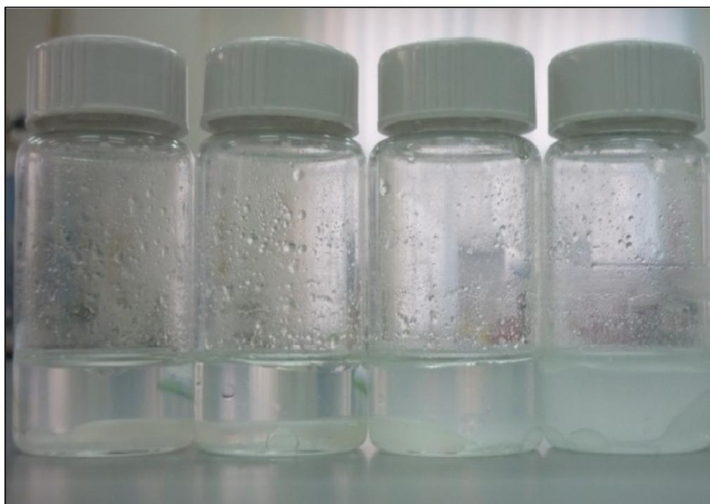
Figure 4.5: Mixture of [Bmim][FAP], Cyanex923 and phenol solution (from left to right: increase in Cyanex923 concentration)
