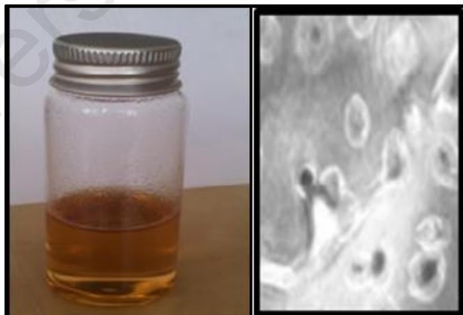
Figure 3.2: The polymer composite solution and its microscopic image
