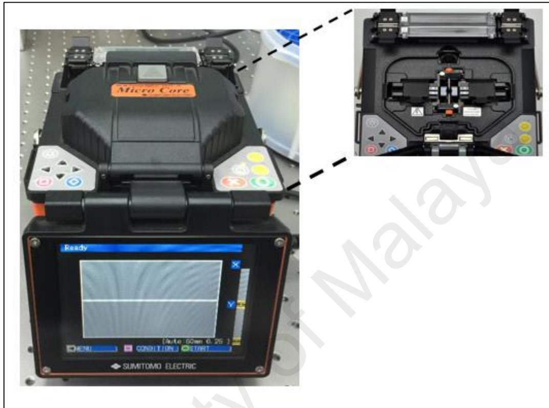
Figure 4.2: The image of a fusion splicer machine (Sumitomo Type 39). Inset shows the image of the working area.
