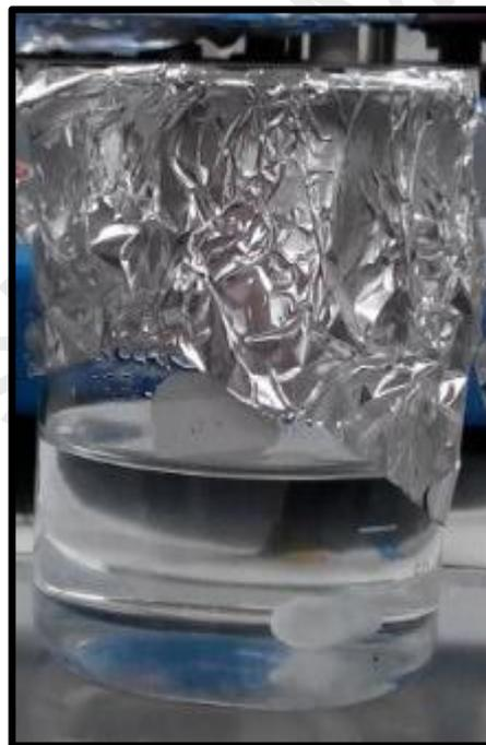
Figure 5.2: The ZnO solution was kept for 24 hours before use
