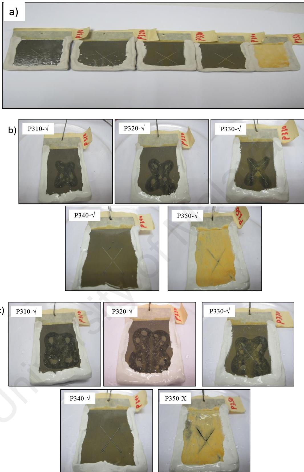
**Figure 7.3:** Acid resistance response for P3 system after a) 0, b) 4, c) 8, d) 15, e) 22 and f) 40 days of immersion in  $H_2SO_4$  10 % solution
