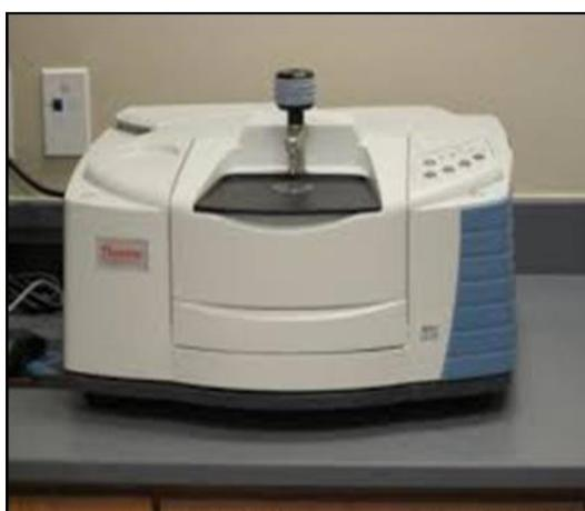
**Figure 3.9:** FTIR Spectrometer (ATR-Nicolet iS10)
