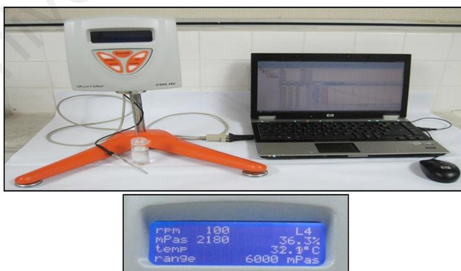
**Figure 3.1:** Elcometer Rotary Viscometer (RV1-L)
