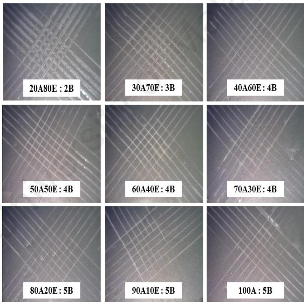
**Figure 4.4:** Cross Cut Images of nAnE Binder System
