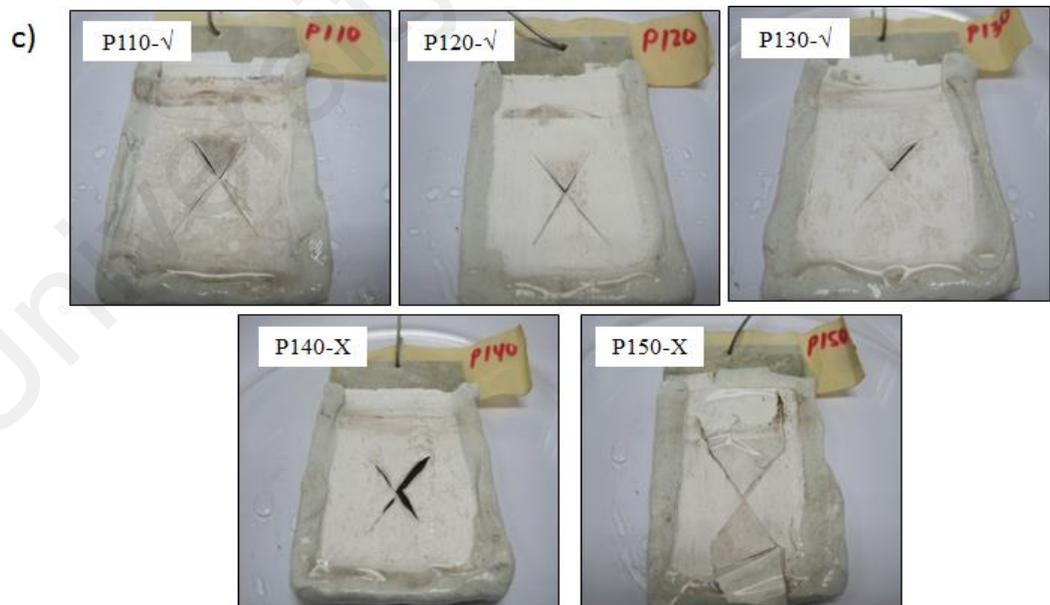
**Figure 7.1:** Acid resistance response for P1 system after a) 0, b) 4, c) 8, d) 15, e) 22 and f) 40 days of immersion in  $H_2SO_4$  10 % solution
