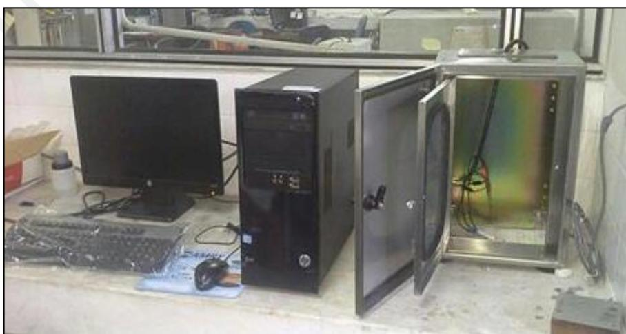
**Figure 3.16:** EIS Instrument with Faraday Cage
