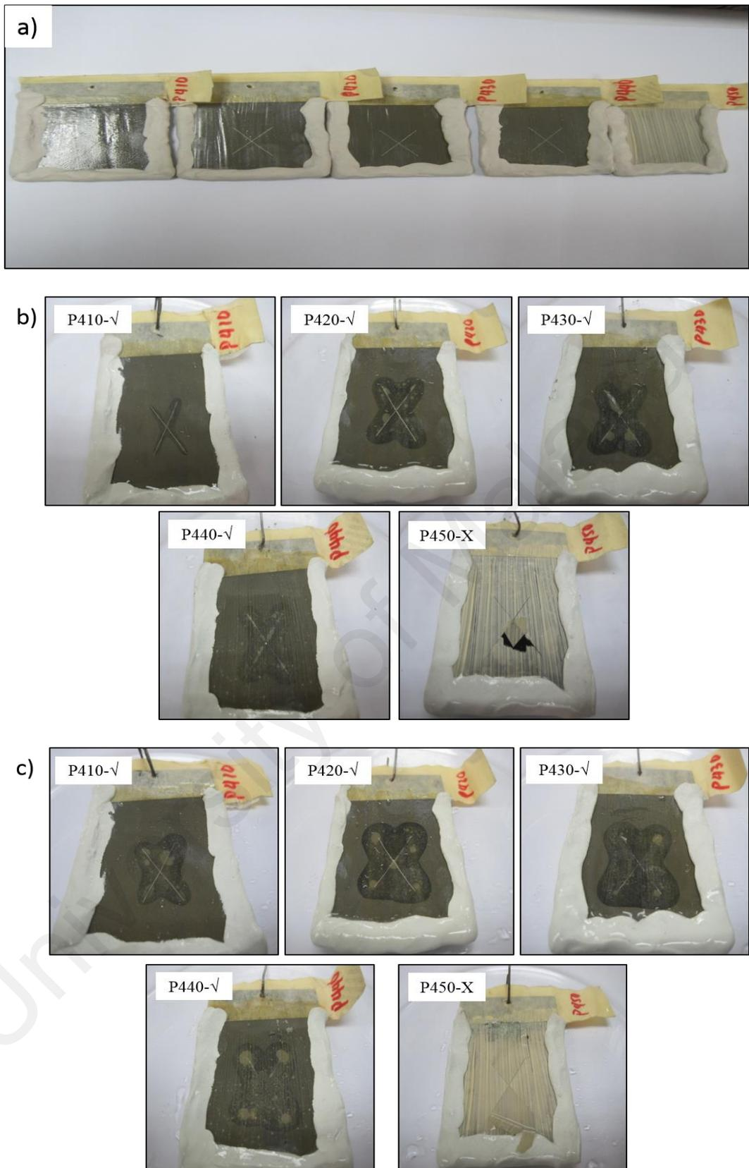
**Figure 7.4:** Acid resistance response for P4 system after a) 0, b) 4, c) 8, d) 15, e) 22 and f) 40 days of immersion in  $H_2SO_4$  10 % solution
