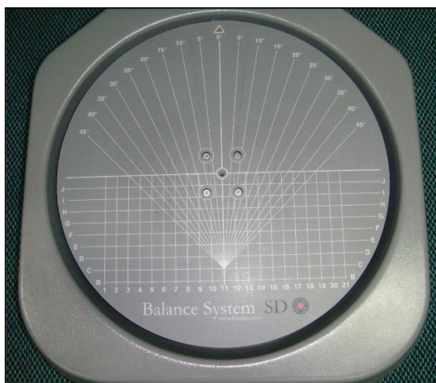
Figure 3.22: The stability platform with adjustable stability level.
