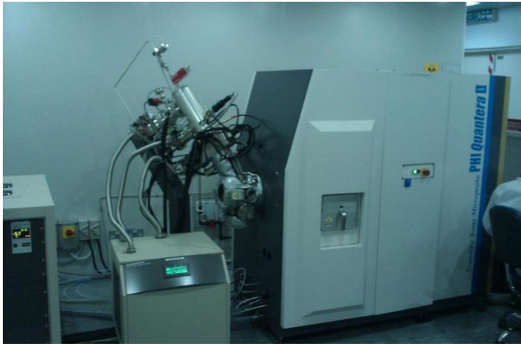
**Figure 3.12: A photograph of PHI Quantera II XPS system.**
