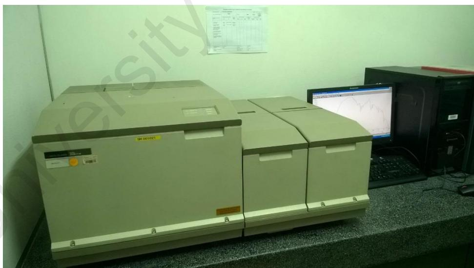
**Figure 3.8: A photograph of FTIR Perkin-Elmer System 2000.**
