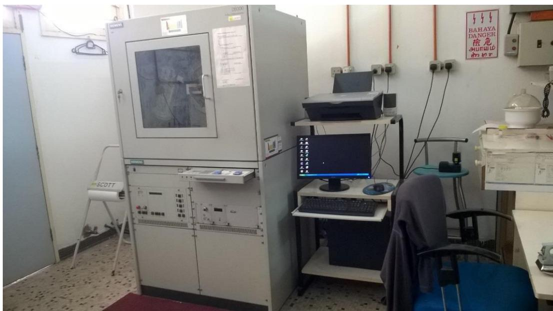
**Figure 3.7: A photograph of SIEMENS D5000 X-ray diffractometer.**
