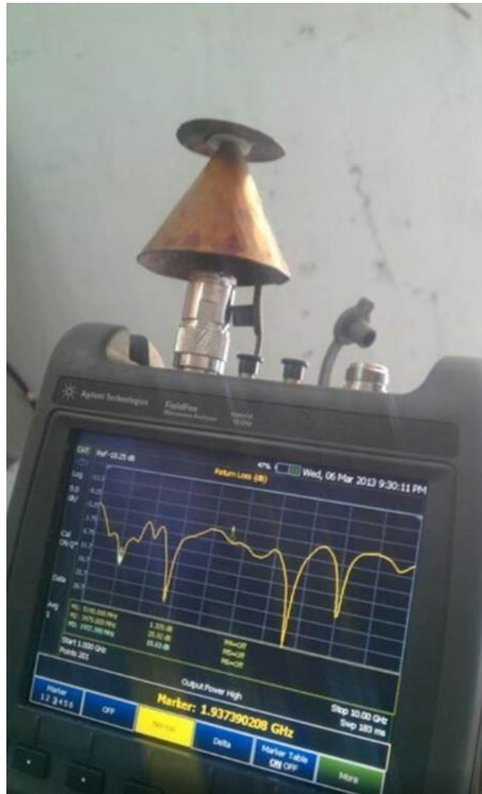
Figure 4.5: Sensitivity of the antenna in the L-Band
