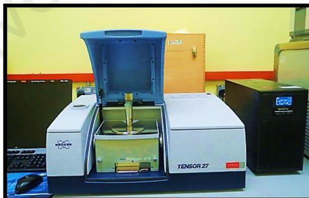
Appendix A.8. Fourier transform infrared spectroscopy (FT-IR, Bruker Tensor 27)
