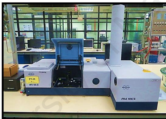
Appendix A.7. Fourier transform infrared spectroscopy (FT-IR, Bruker IFS 66/S)
