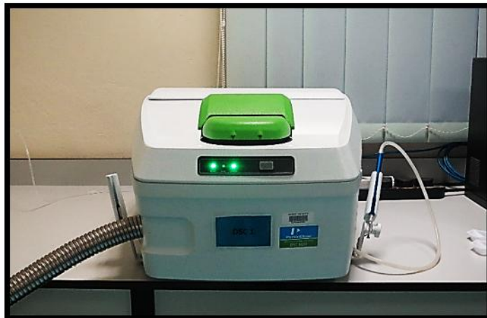
Appendix A.6. Differential Scanning Calorimetric (DSC, Perkin Elmer DSC 8000)
