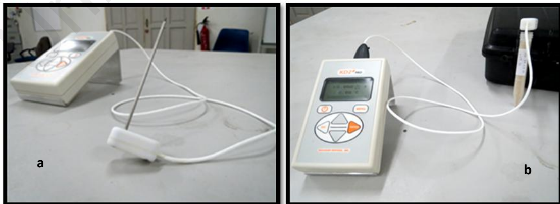
Appendix A.5. KD2Pro measurements; a) single needles sensor (TR-1); b) measurements setup
