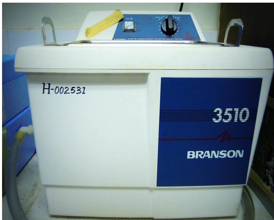
Figure 3.5: Ultrasonic cleaning bath used for sonication
