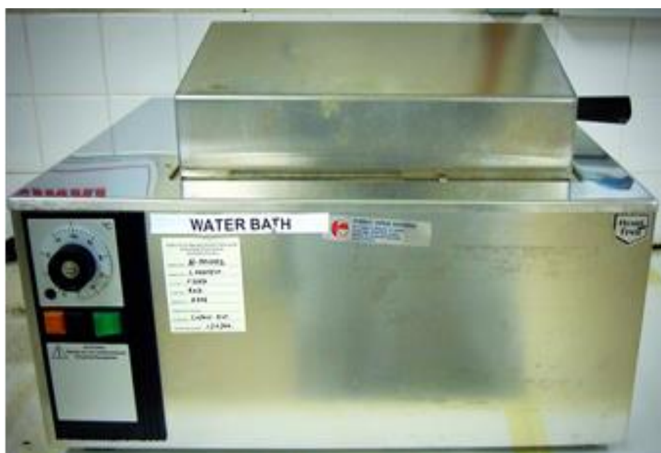
Figure 3.2: Covered water bath used for thermal treatment
