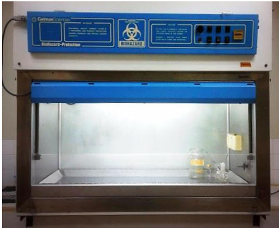
Figure 3.7: UV-C lamp in a laminar flow cabinet
