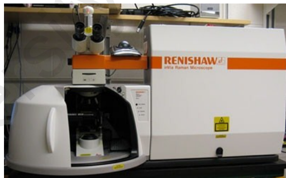
Figure 3.11 :Renishaw in Via Raman Microscope.
