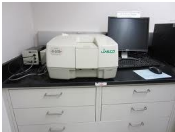
Figure 3.5 :Jasco V-570 UV/VIS/NIR Spectroscopy
