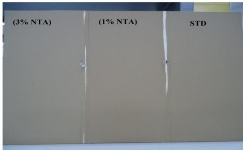
Fig. 4.5 Degree of chalking indication for NP Weatherbond Deep Base tinted for all three specimens
