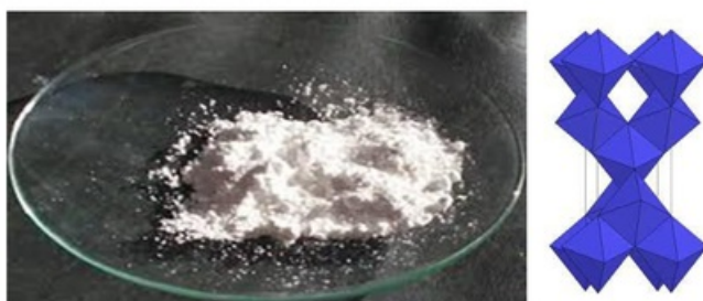
Fig.2.1 The powder form of Nano \text{TiO}_2 and the anatase structure of the material.
