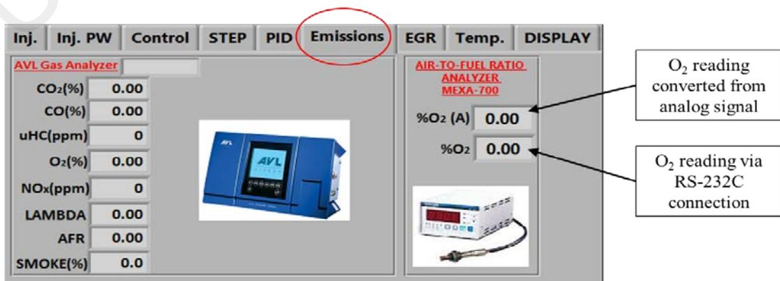
**Figure 3.40:** MEXA-700λ O<sub>2</sub> reading interface program tab.
