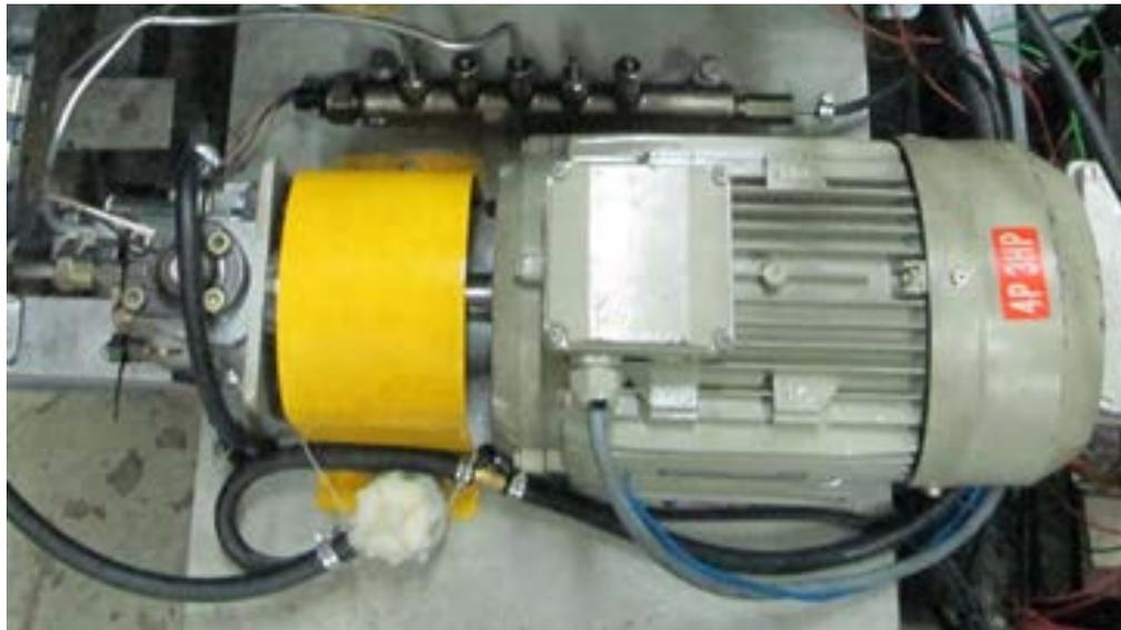
**Figure 3.5:** Fuel delivery setup with pump driven by electric motor.
