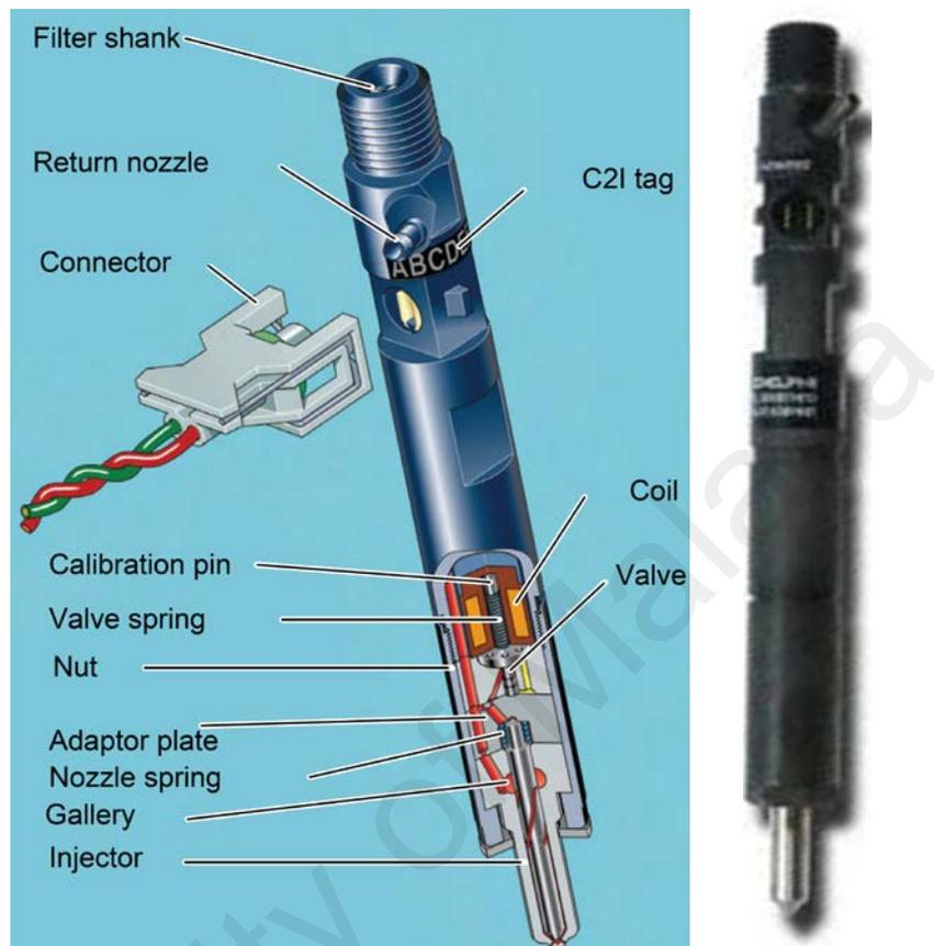
**Figure 3.18:** Diesel solenoid injector (Delphi France SAS, 2007).
