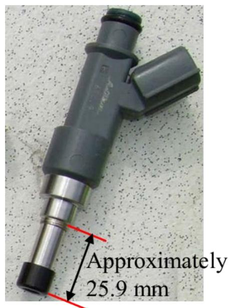
**Figure 3.19:** Denso port fuel injector.
