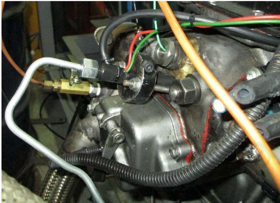
**Figure 3.20:** Common-rail injector mounted on the engine cylinder head.
