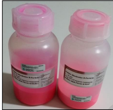
Figure 3.13 : Fluorescent Particles (Seeds) of two sizes from Dantec Dynamic
