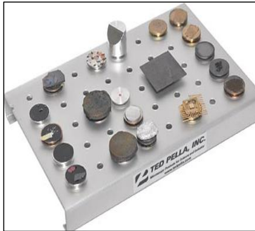
Figure 2.12 : Different models of specimen with metals coated (Ted Pella, 2014)
