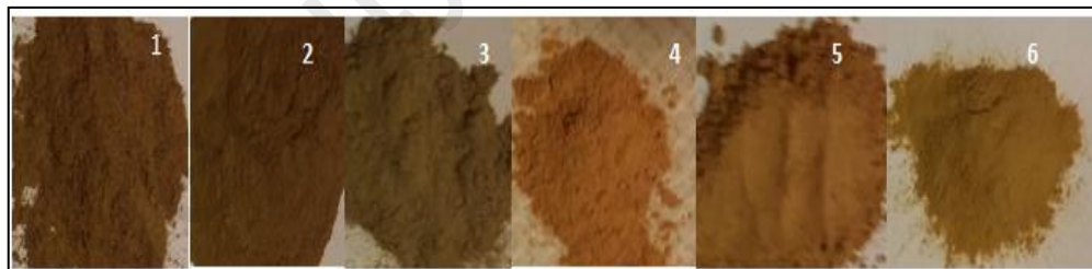
Figure 3.2 : Images of the sieved ( <63\ \mu\text{m} ) soil samples: 1/Sample 1 Loamy sand, 2/sample 2 Sandy loamy clay, 3/Sample 3 Sandy clay loam, 4/Sample 4 Clay, 5/Sample 5 Clay, 6/Sample 6 Sandy Clay.
