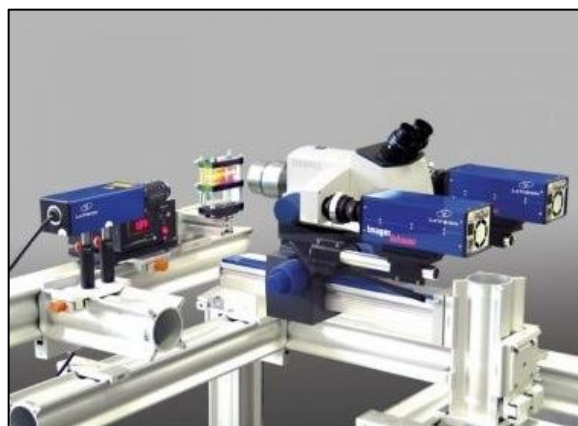
Figure 2.26 : Schematic of Micro-PIV(Lavision, 2014)
