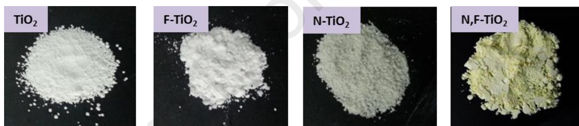
Figure 4.30: Appearance (color) of un-doped TiO 2 , F-TiO 2 , N-TiO 2 and N,F-TiO 2
