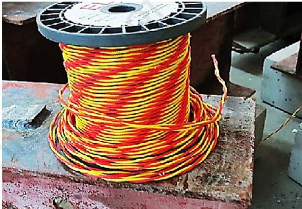
Figure 3.9: Cable thermocouples type K for measuring the temperature in the specimens
