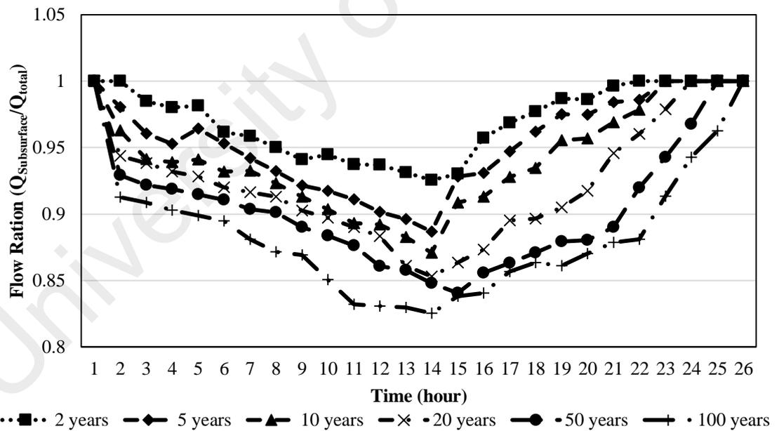
Figure 4.25: Subsurface flow ratio during 24 hours rainfall events with different ARI
