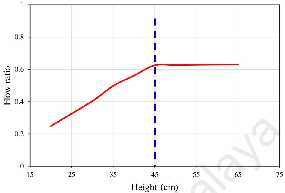
Figure 4.29: The determination of optimum size for subsurface conduit module for rainfall event 2
