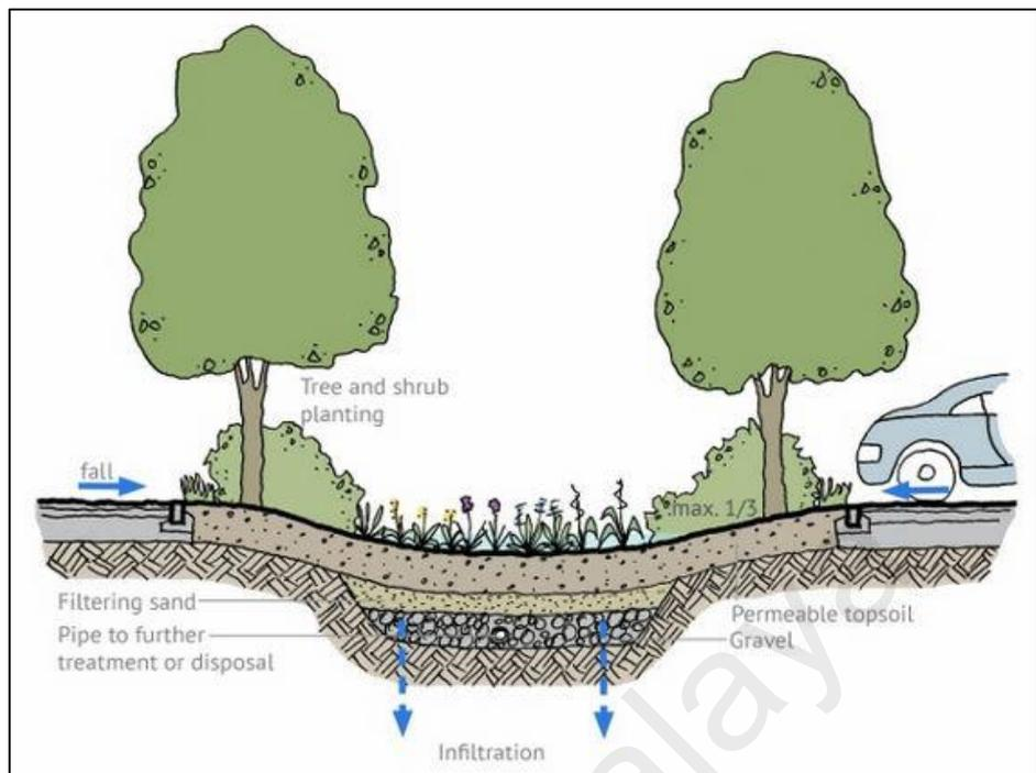
Figure 2.10: Sample of constructed Bioretention (CIRIA, 2007)
