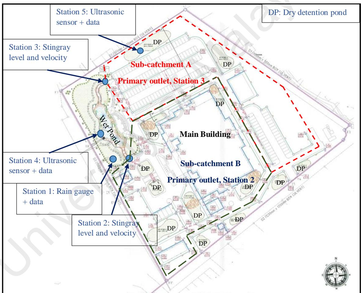
Figure 3.8: Plan view of study area and location of rainfall-runoff monitoring stations
