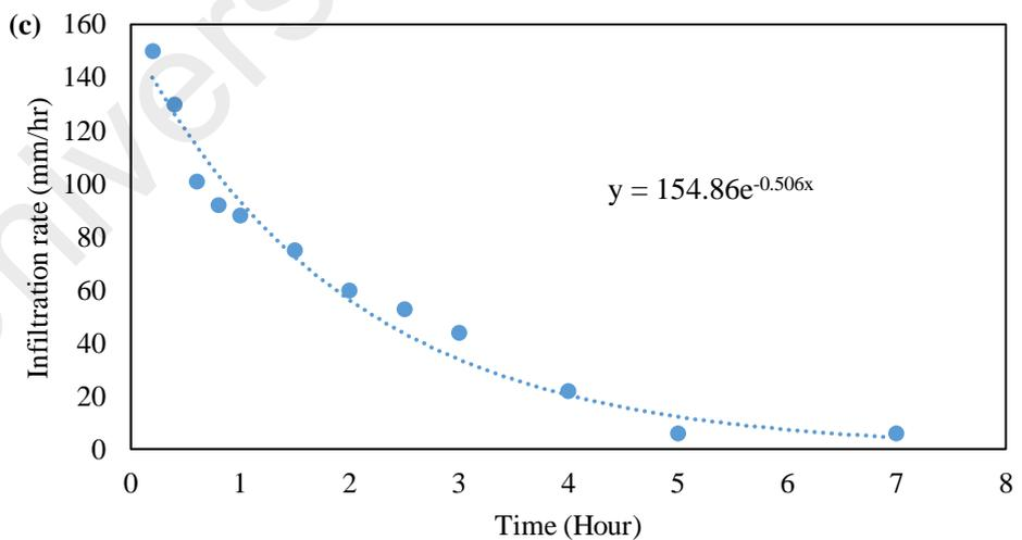
Figure 4.8: Conducted infiltration test: (a) Dry pond without detention storage, (b) Dry pond with detention storage, (c) Grass swale
