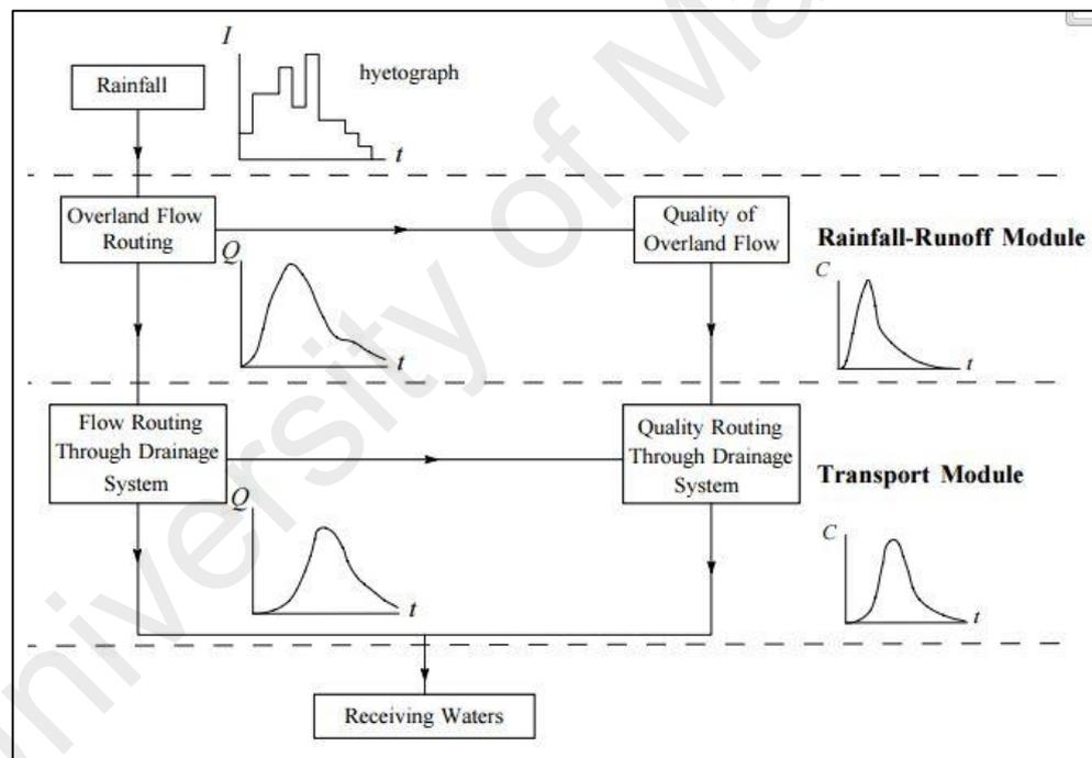
Figure 2.24: Overview of processes incorporated in Urban Stormwater Model (Nix, 1991; Zoppou, 2001)
