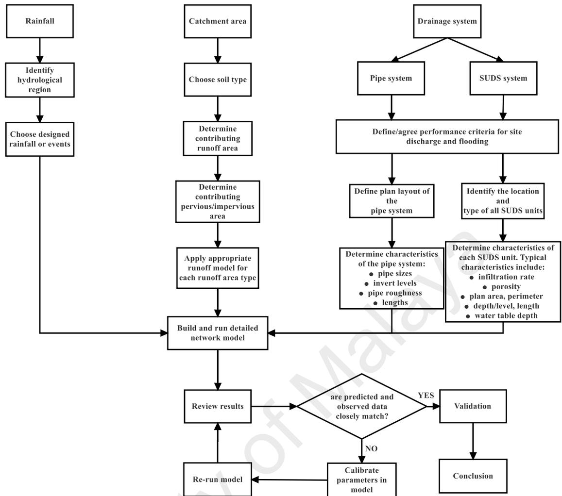
Figure 3.15: Processes for modelling urban drainage system in InfoWorks SD
