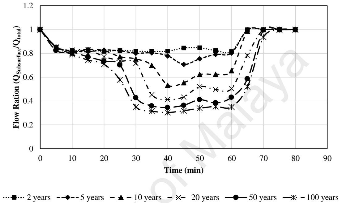
Figure 4.23: Subsurface flow ratio during 1 hour rainfall events with different ARI
