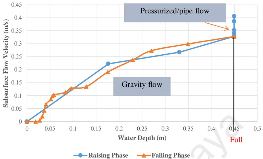
Figure 4.30: Flow characteristics for subsurface conveyance system for rainfall event 5
