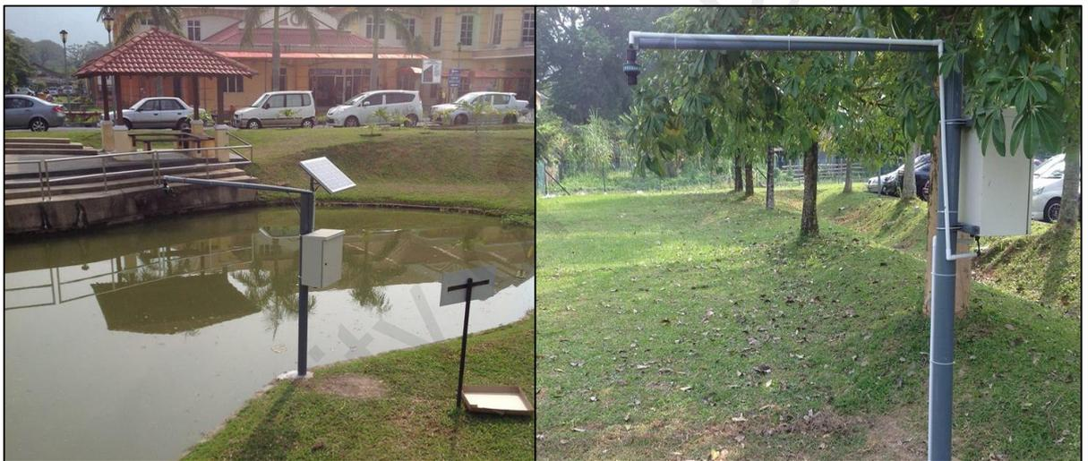
Figure 3.11: Ultrasonic sensor to measure water level in Retention pond (Left) and dry detention pond (Right)
