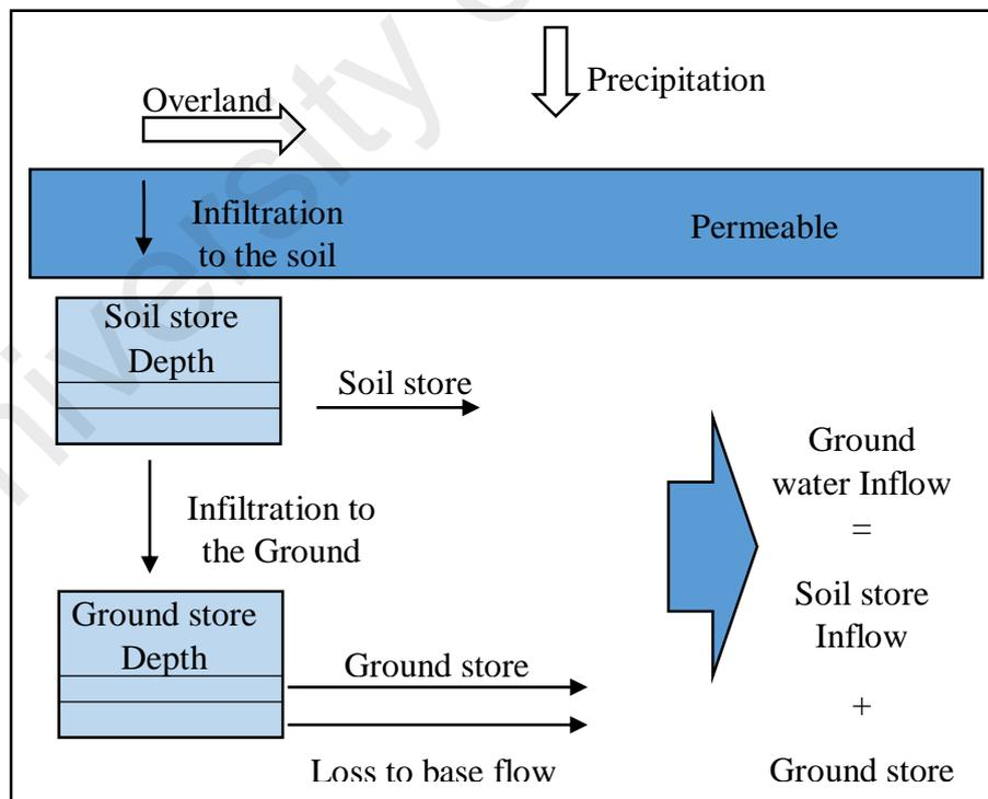
Figure 3.16: Integrated rainfall-runoff model in InfoWorks SD
