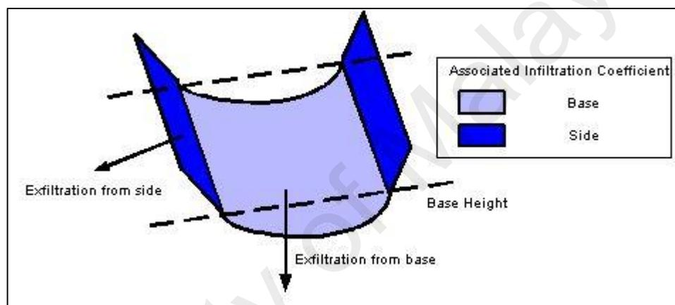
Figure 3.17: schematic plan of required parameters in modelling swale
