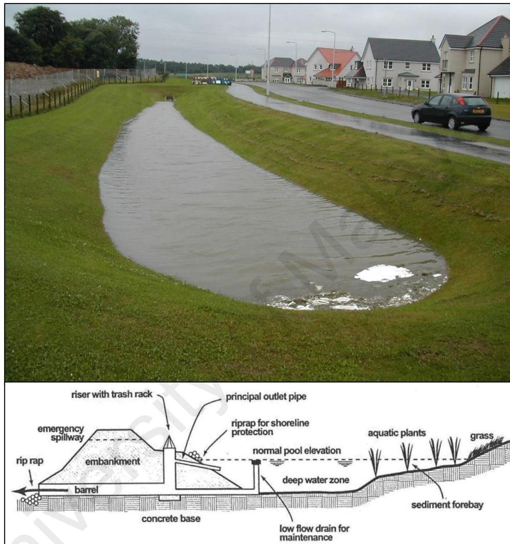
Figure 2.20: Cross sectional design and Dry Detention
