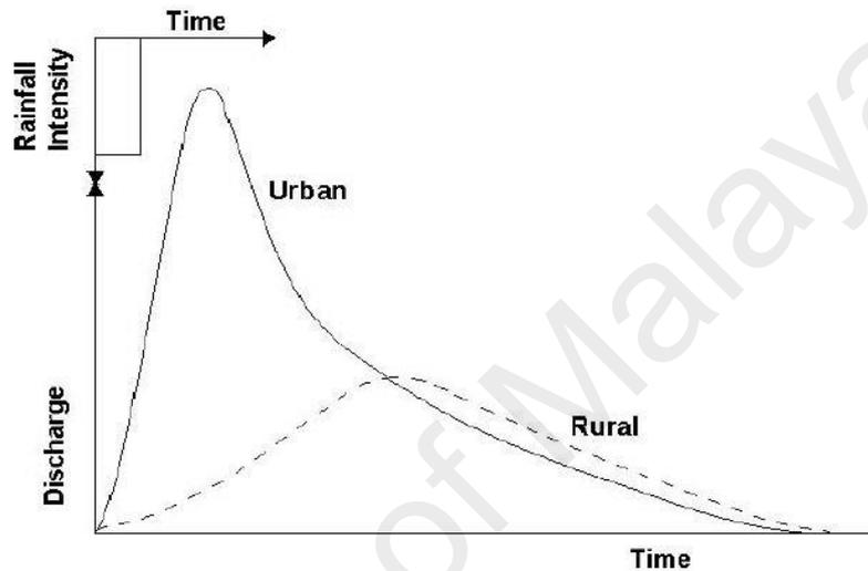
Figure 2.1: Impact of urbanization on runoff quantity (Ramachandra and Mujumdar, 2009)
