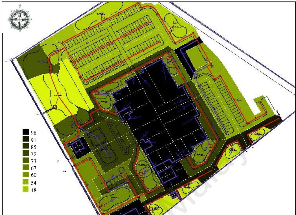
Figure 4.7: CN values for individual subcatchment for study area
