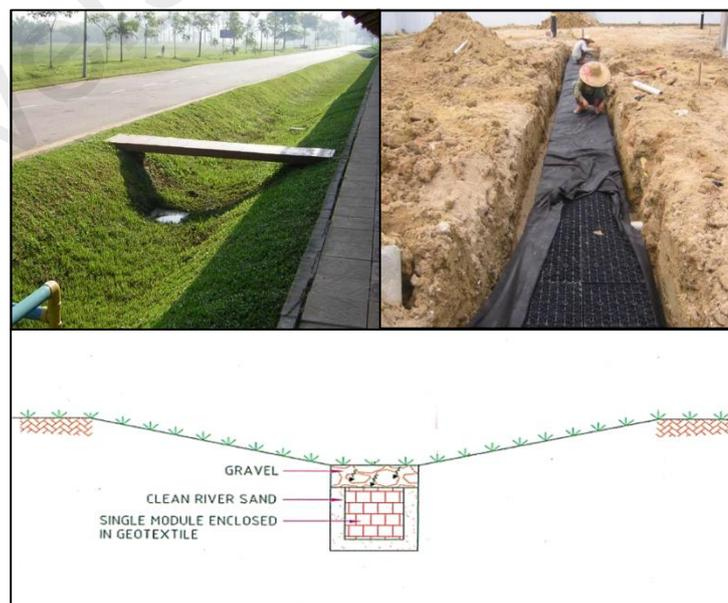
Figure 2.18: Cross sectional profile of grass swale in BIOECODS project (REDAC, 2005)
