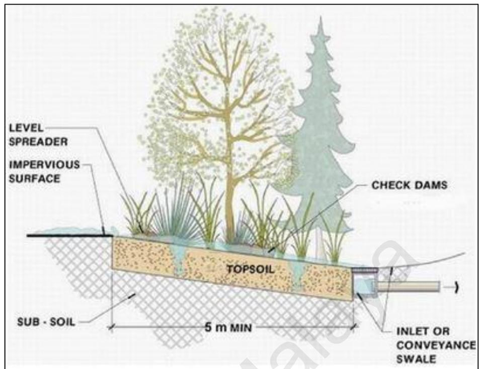
Figure 2.8: vegetated Filter strip (Landmark Design Group)
