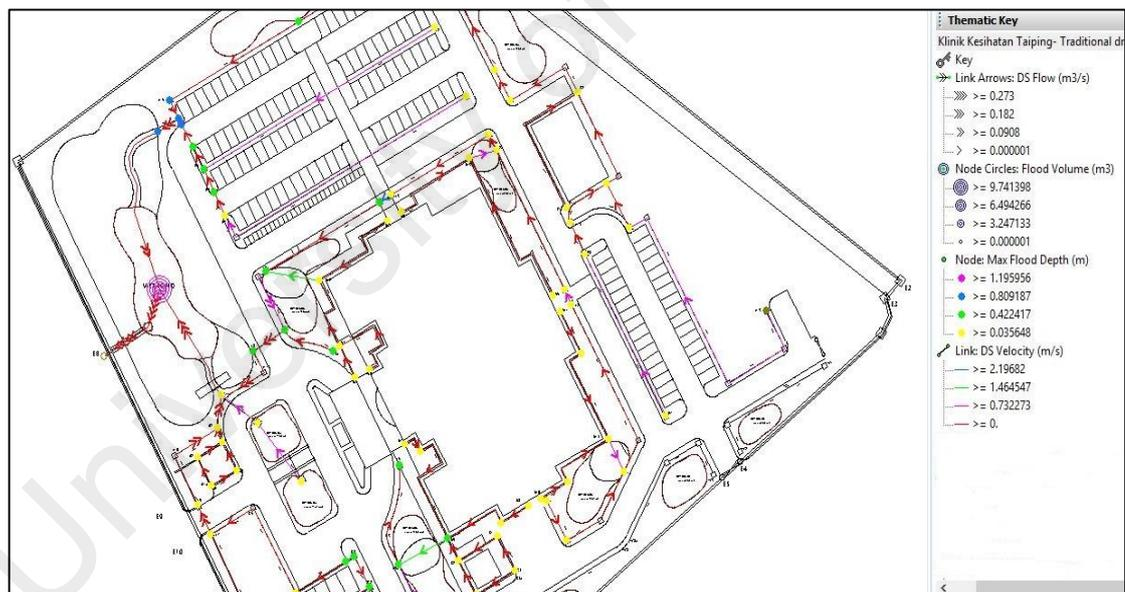
Figure 4.17: Flow simulation (traditional drainage system) for event NO.1 using InfoWorks SD
