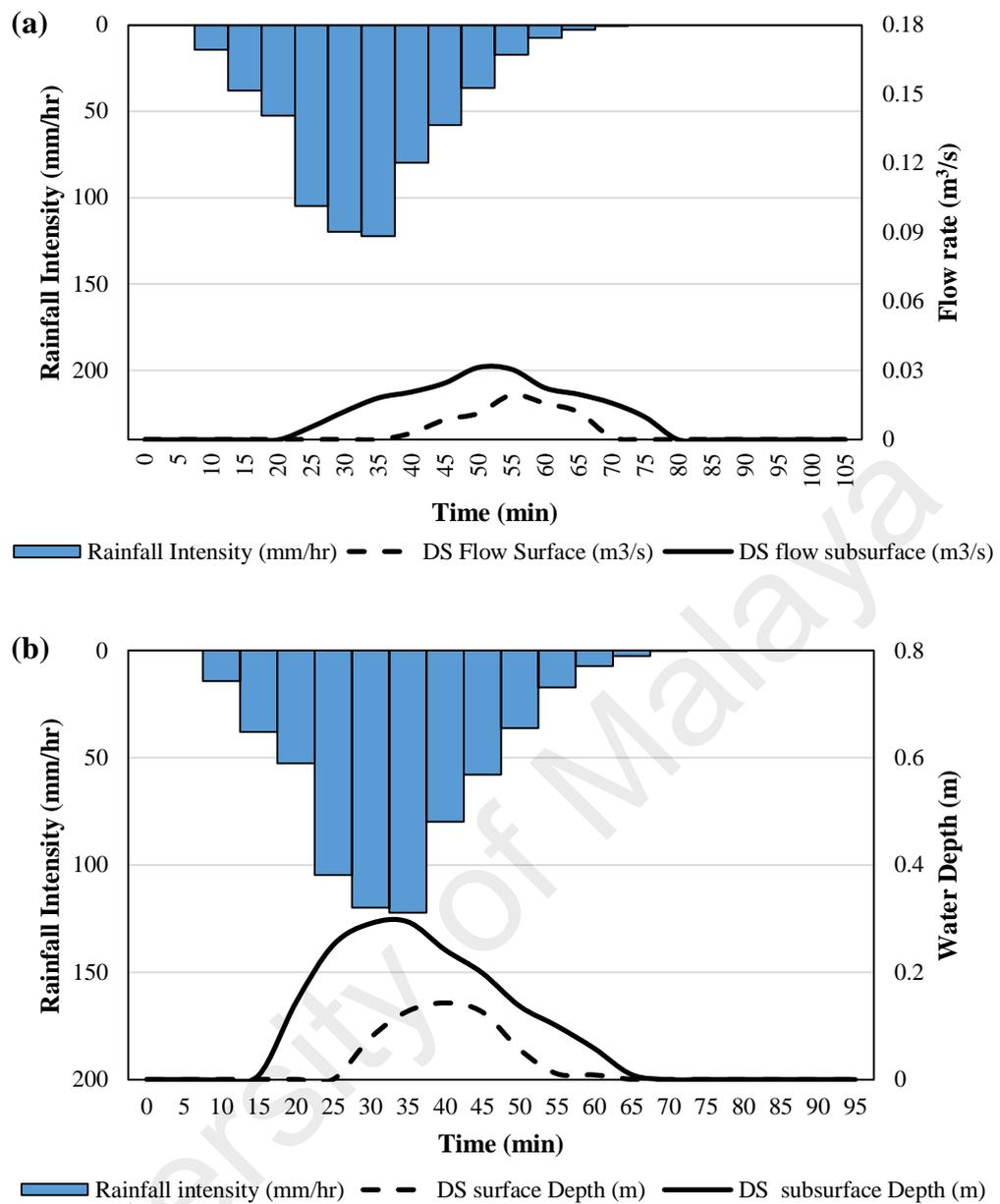
Figure 4.21: Simulated result for high intensity rainfall event No.5 (12/1/2014) in primary outlet monitoring station No.3: (a) Flow rate, (b) Water depth
