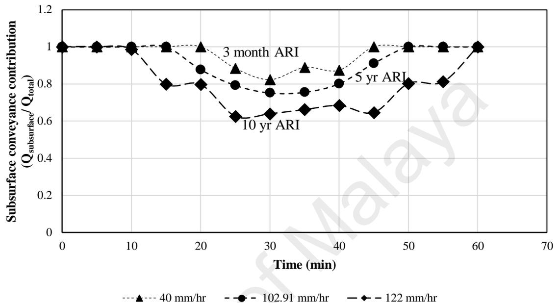
Figure 4.22: Subsurface flow ratio ( $Q_{\text{Subsurface}}/Q_{\text{total}}$ ) during rainfall events with different intensity and patterns
