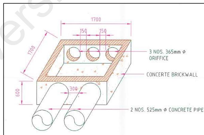
Figure 3.4: Designed outlet structure for wet pond in study area (Source: JKR, 2005)
