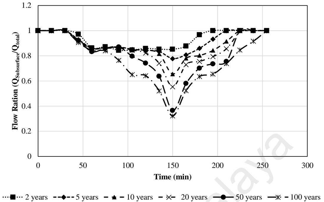
Figure 4.24: Subsurface flow ratio during 3 hours rainfall events with different ARI
