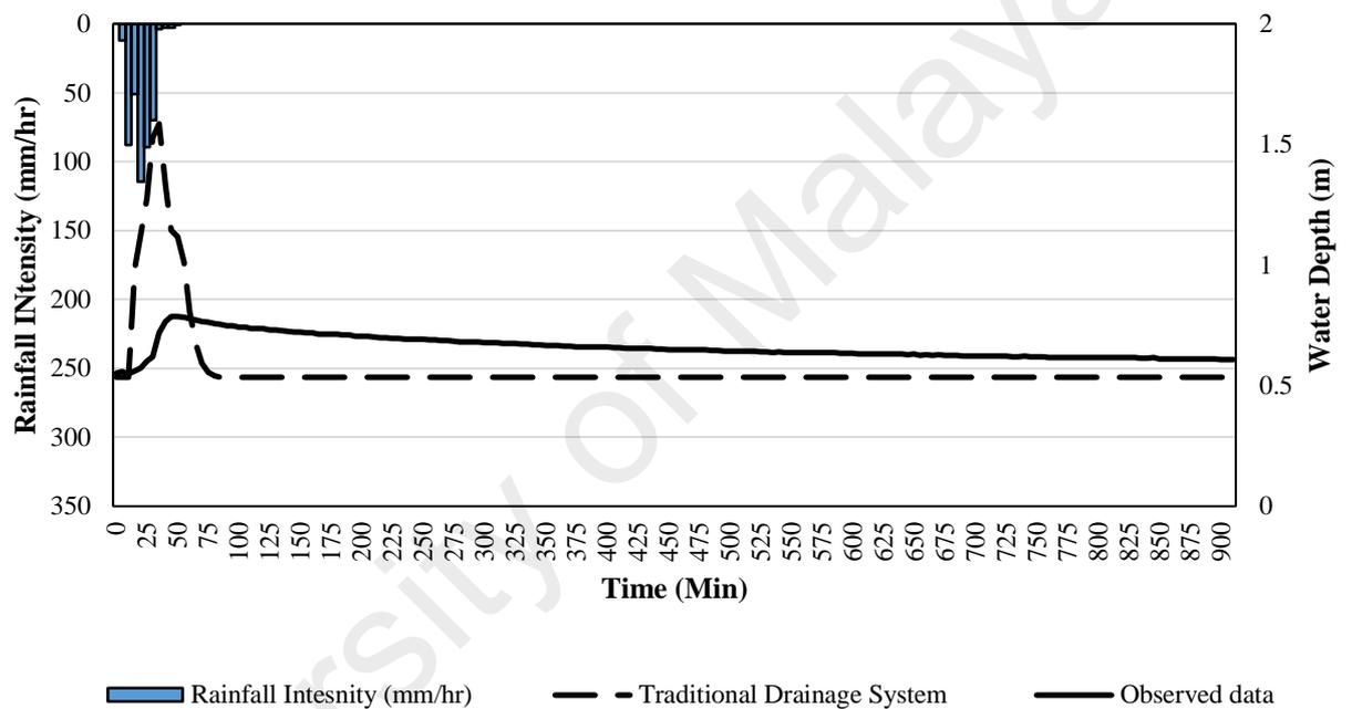
Figure 4.28: Comparison of modelled traditional drainage system and observed water level in downstream (retention pond) for rainfall event number two (14/10/2013)
