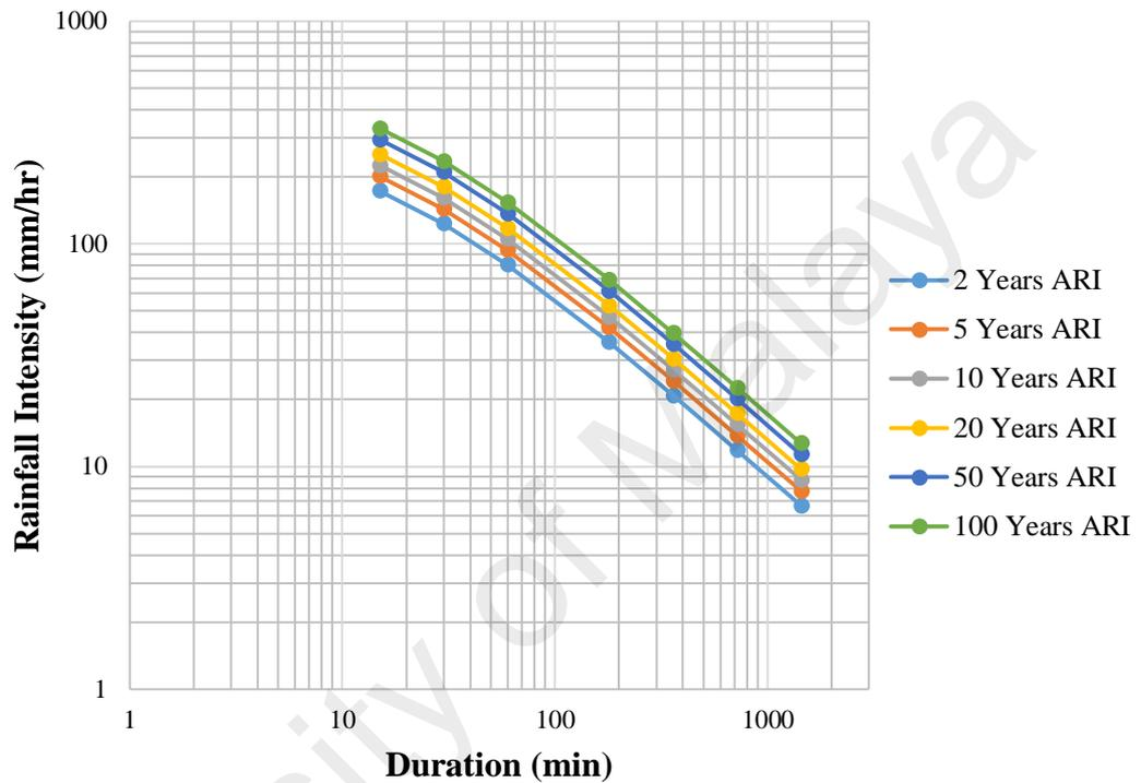
Figure 4.12: IDF Curve for Taiping, Perak
