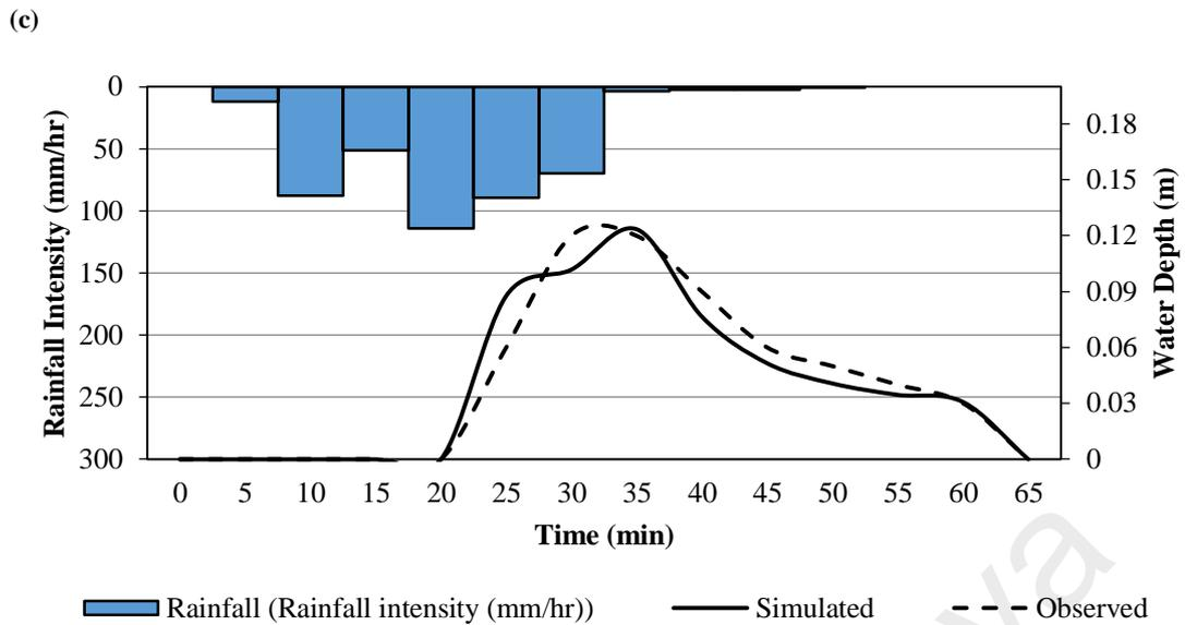
Figure 4.13: Comparison of modelled (BIOECODS) and observed water level for rainfall event 14/10/2013, (a) Retention pond station No.4, (b) Primary outlet station No. 3, (c) Primary outlet station No.2
