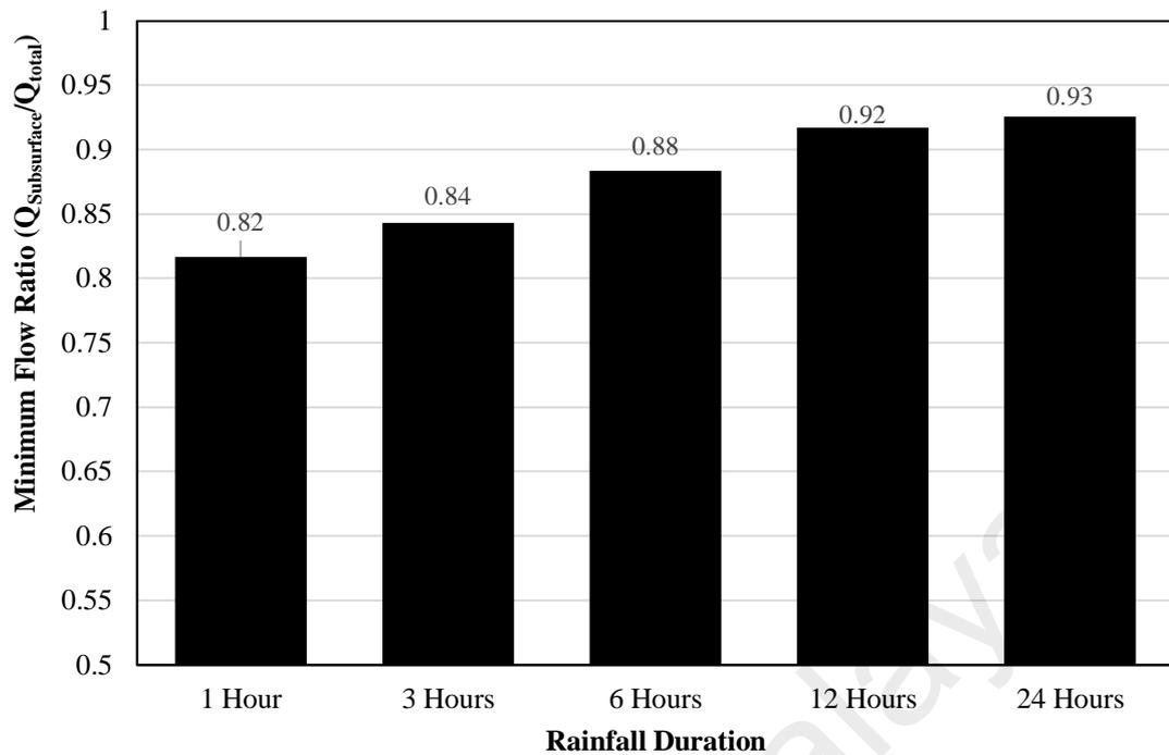
Figure 4.27: Minimum contribution of online subsurface conveyance system in different rainfall duration with 2 years ARI
