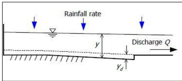
Figure 2.22: Definition of Non-linear Reservoir method (MSMA, 2001)
