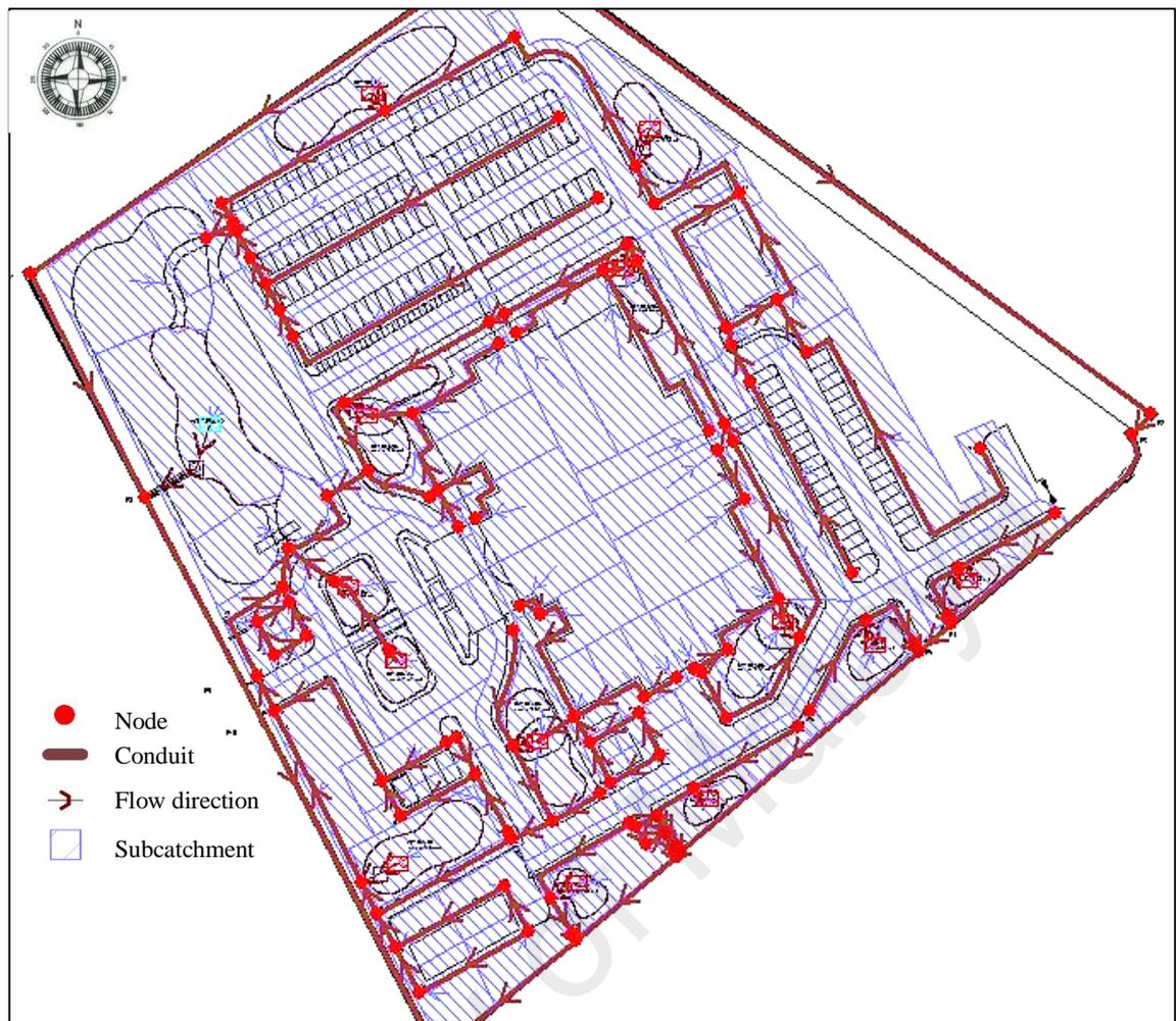
Figure 4.4: Drainage network and subcatchments map for BIOECODS system modelled in InfoWorks SD
