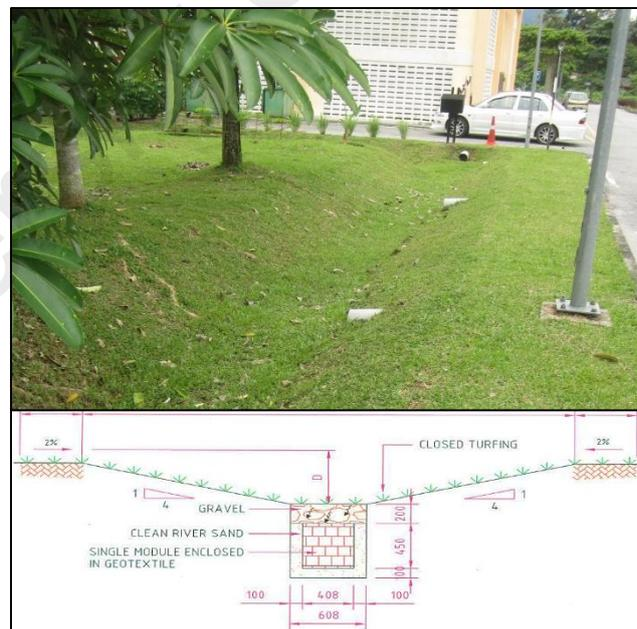
Figure 3.6: Design plan of constructed grass swale with on-line subsurface conveyance
