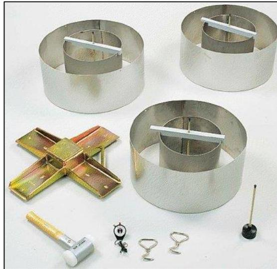
Figure 3.12: Double-ring parts for infiltration test
