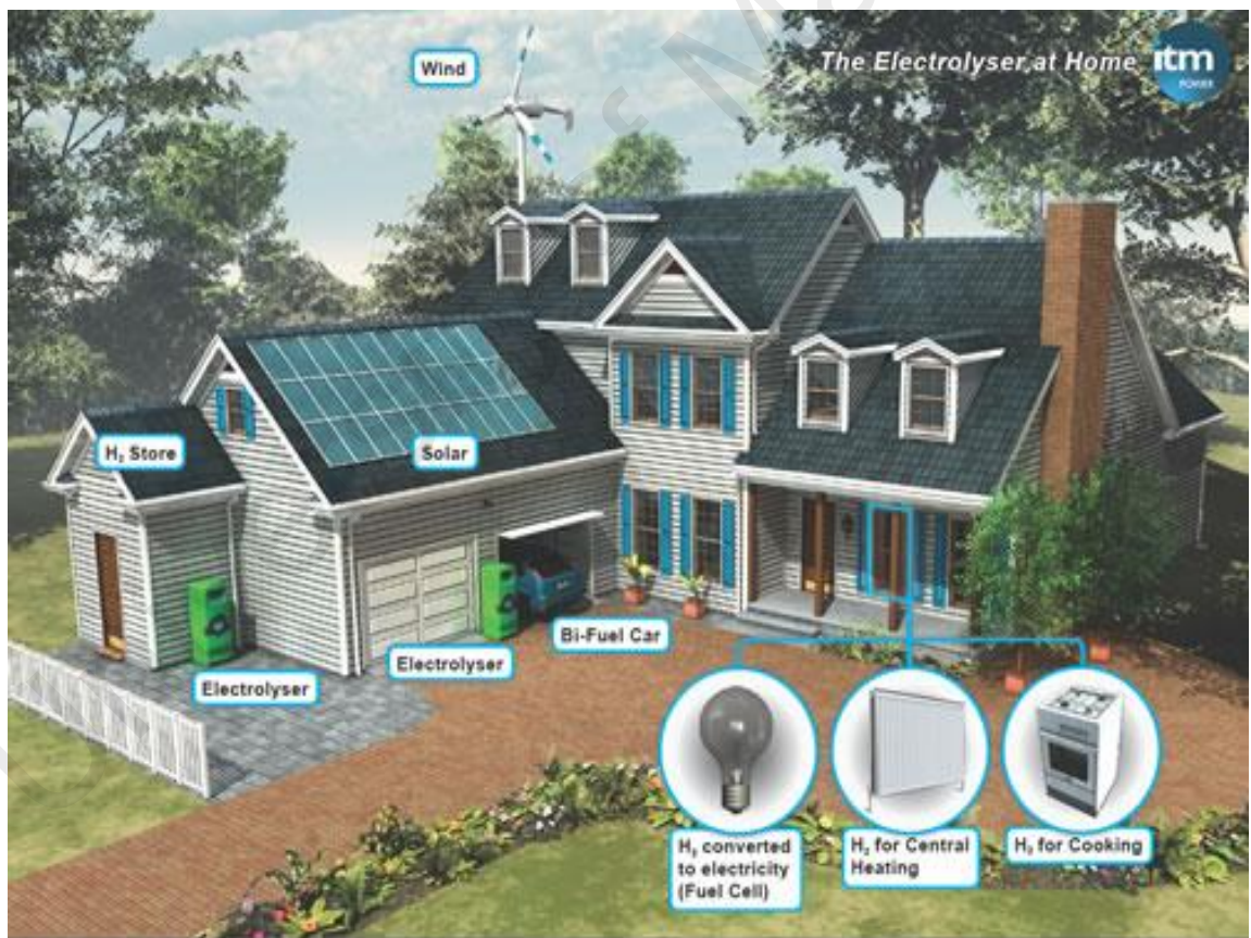
Figure 2.10: Fuel cell used in a residential building (source: http://www.cleantechinvestor.com/portal/interviews/1765-the-hydrogen-home.html )
