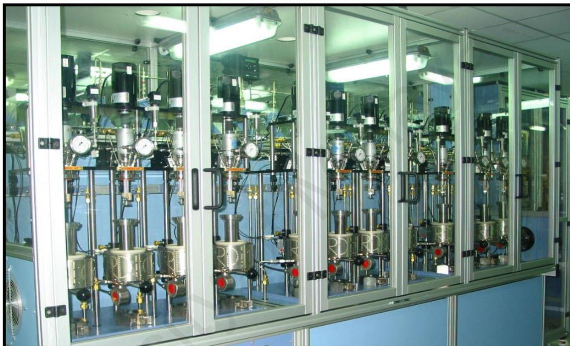
**Figure 3.6: A workstation that consist 12 independent batch reactors**
