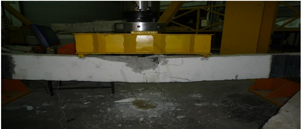
Figure 4.10: Flexure failure mode of H1B8S19L73W2TAS
