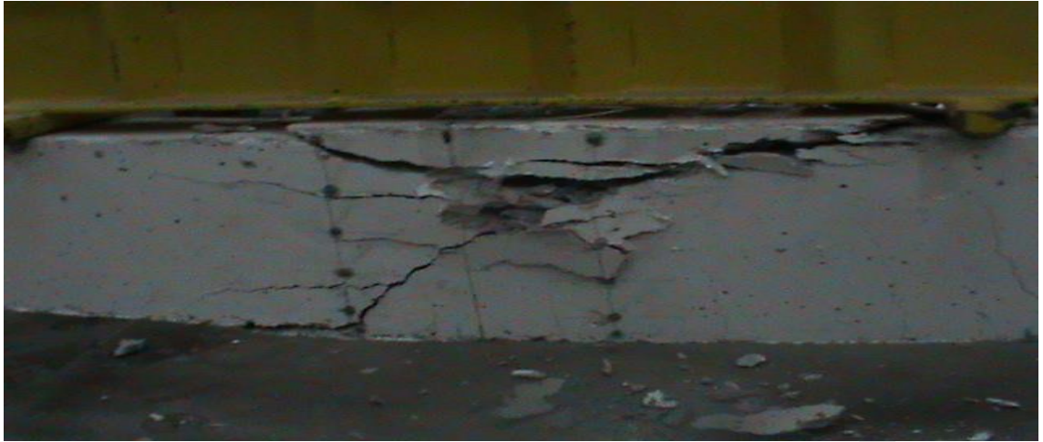
Figure 4.9: Flexure failure mode of H2B6S19L125W1.5T
