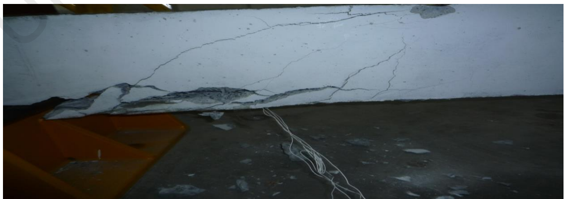
Figure 4.23: Debonding failure mode of H1BP8F16L80W1.2T
