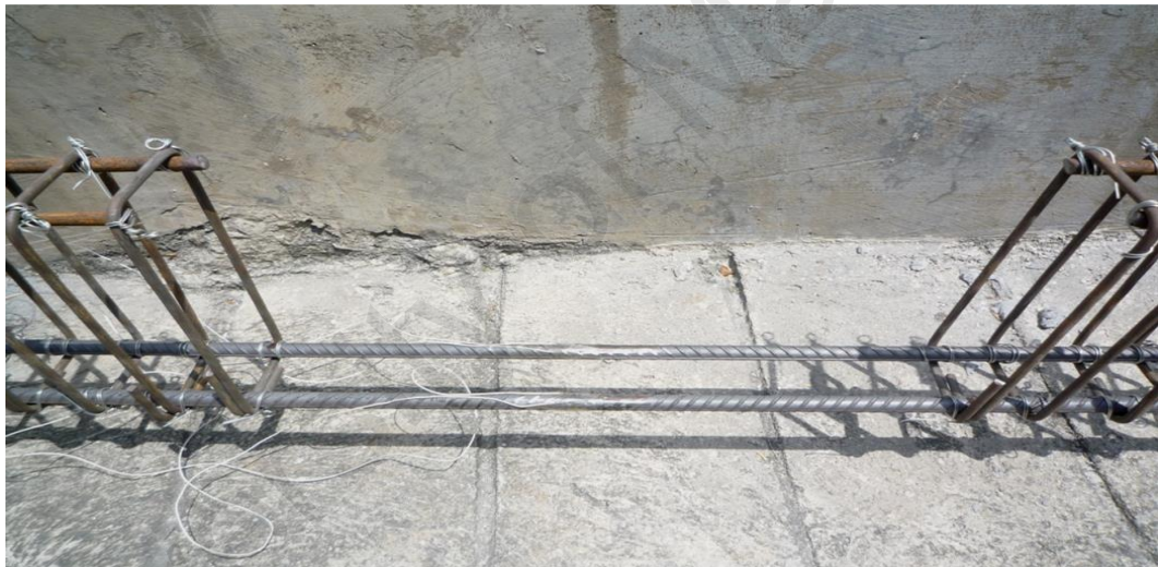
Figure 3.9: Attachment of strain gauges
