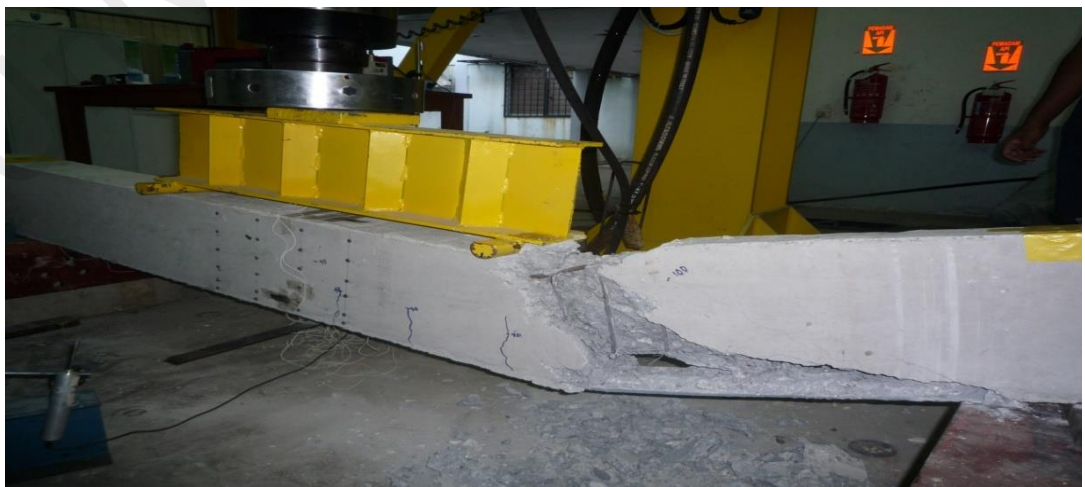
Figure 4.5: Debonding failure mode of H2B6S19L73W2T
