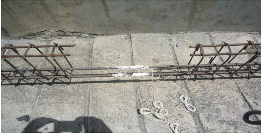
Figure 3.10: Strain gauges covered with silicone gel
