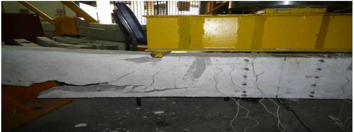
Figure 4.24: Debonding failure mode of H1BP6F16L80W1.2T
