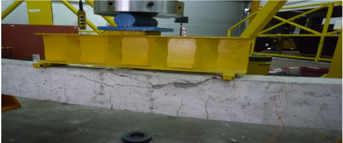
Figure 4.41: Failure mode of N1S8C
