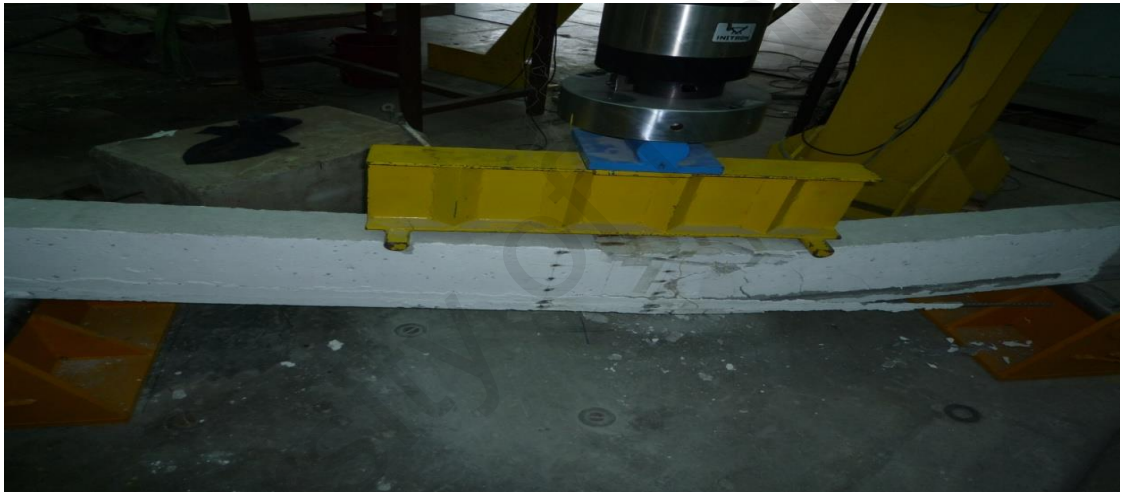
Figure 4.42: Failure mode of N3S8C
