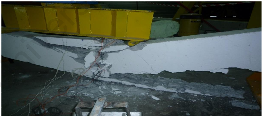
Figure 4.2: Debonding failure mode of H1B8S16L73W2T
