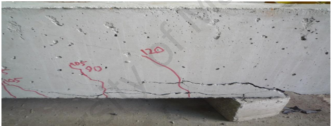
Figure 4.25: Debonding failure mode of H2BP6F16L80W1.2T
