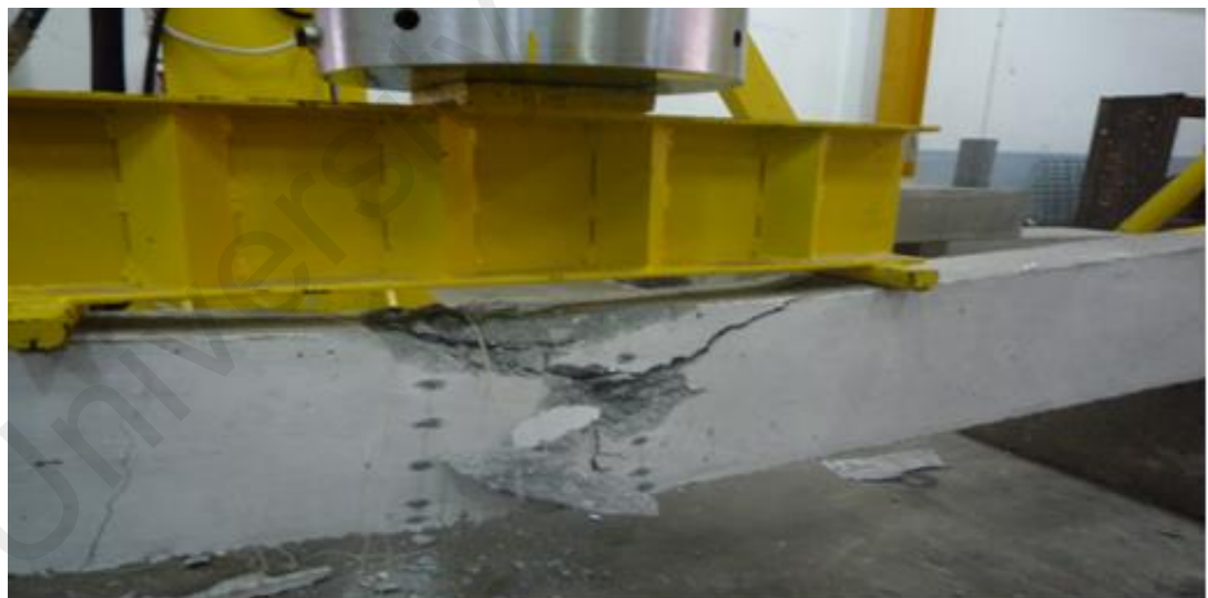
Figure 4.37: Failure mode of N2S6C
