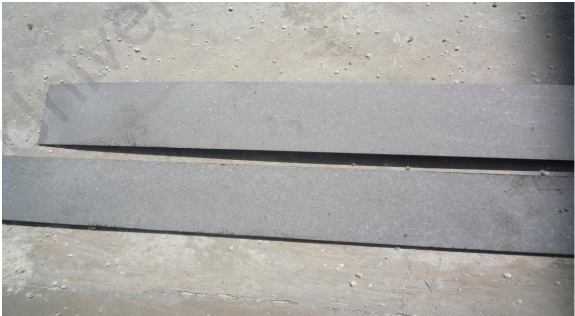
Figure 3.5: Sand blasted steel plate
