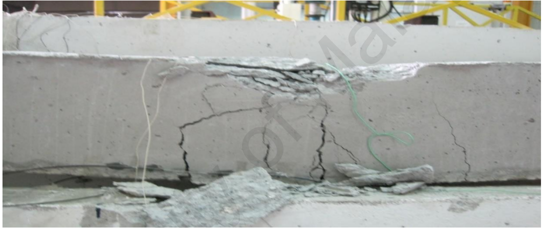
Figure 4.39: Failure mode of N2S6EC
