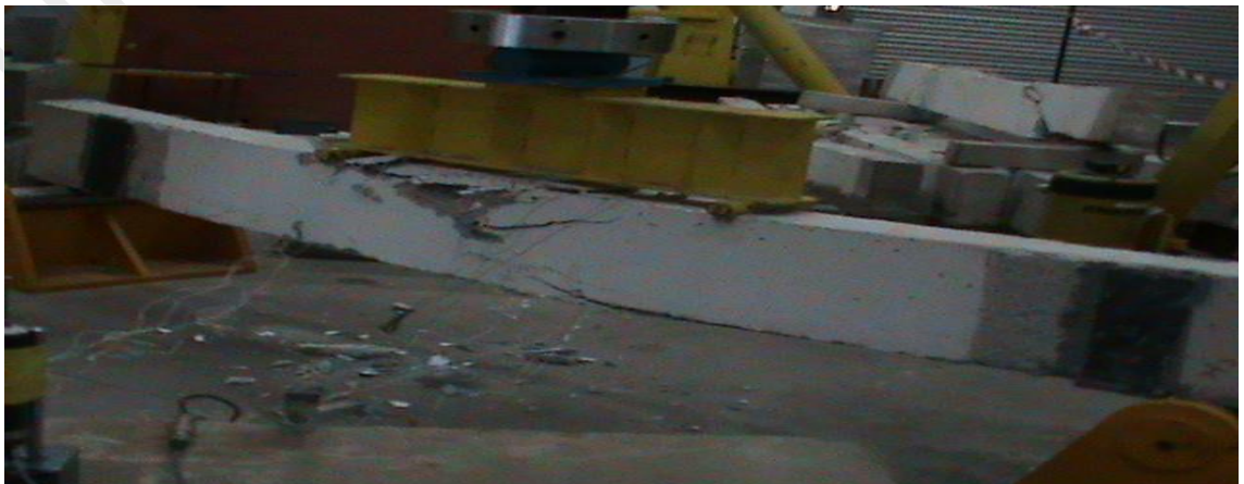
Figure 4.26: Flexure failure mode of H1B8F19L80W1.2TAF
