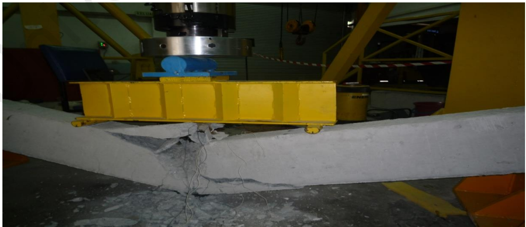
Figure 4.40: Failure mode of N1S8E
