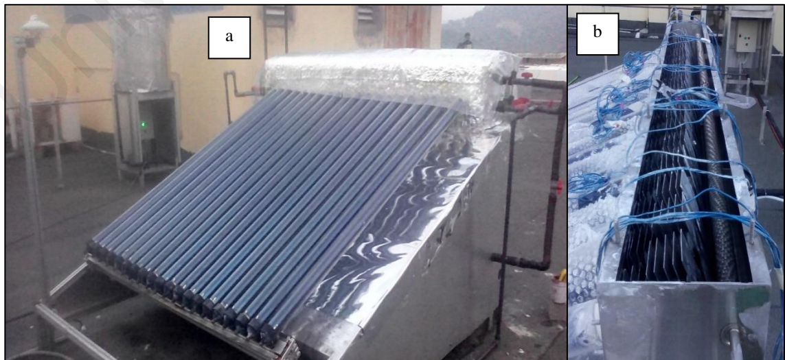
Figure 3.13: a. Photo of HPSC-LHS experimental setup, b. Photo of inside of the LHS tank.
