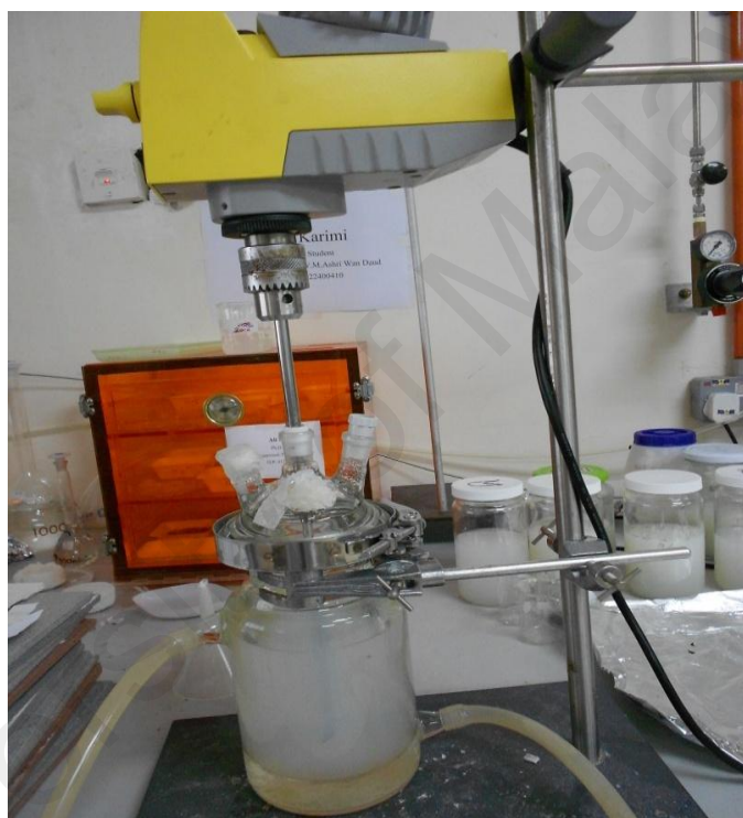
Figure 3.2: Setup for synthesis of PVA/ Na + -MMT nanocomposite hydrogels
